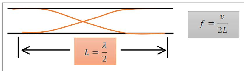
**Figure 7:** The fundamental or first harmonic of open resonance tube
