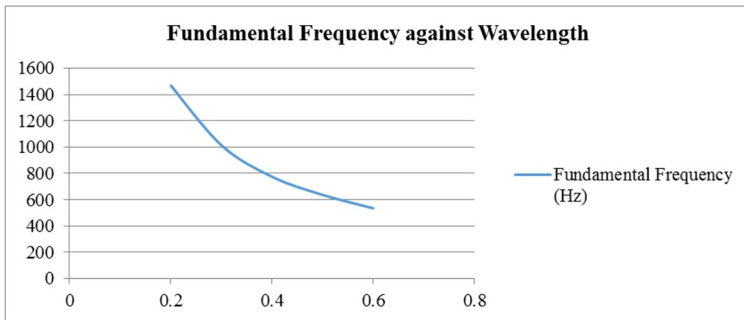
**Figure 10:** Graph of fundamental frequency against wavelength for open resonance tube
