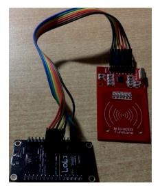
Figure 6. The physical realization of WiRF reader.
