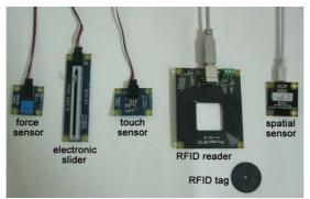
Figure 4. Sensor devices deployed in GraspLearn
