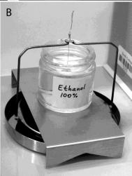
FIGURE 1. A) Specific gravity apparatus mounted in a precision analytical balance.
