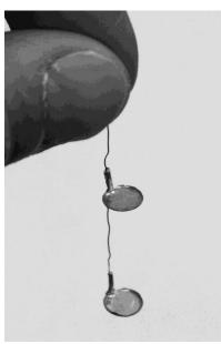
FIGURE 5. Close-up of the double weighing pan assembly.
