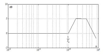
Figure 9. Conditions constraining the relative model error in the case of two unstable zeros
