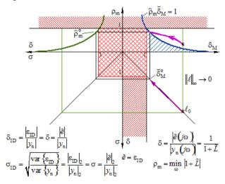
Figure 18. Relationship between the control and identification error in the case of the *KB*-parameterized identification method
