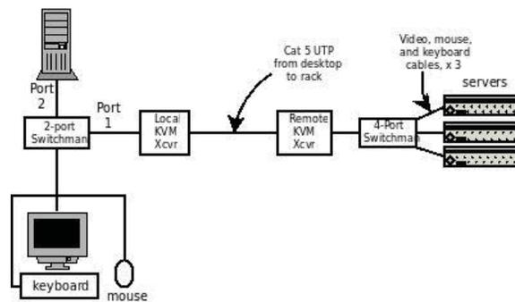
Illustration 2: KVM Switch Wiring. The local switch selects the local workstation (port 2) or a KVM transceiver (Port 1). Special key-strokes enable the user to select any one of three servers attached to the remote 4 port KVM.
