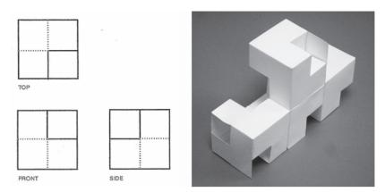
*Figure 2. Four cubic paper models constructed from an orthographic drawing - placed in adjacent relation. (model constructed by Kevin Bates) Source: Stephen Temple*
