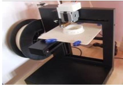
**Figure 2.** Housing for functional speaker 3D printed by first year student, Troy Baverstock.
