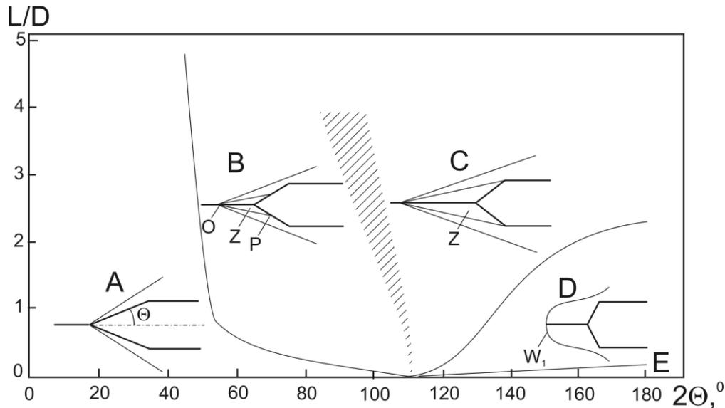
**Figure 1.** Wood's classification of flow types over spiked cone bodies.
