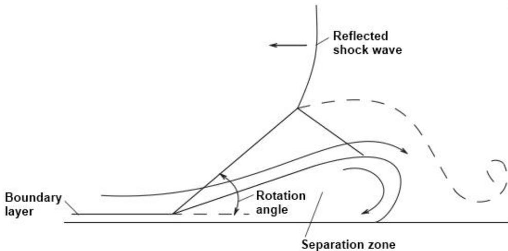
**Figure 3.** The problem of shock wave and boundary layer interaction
