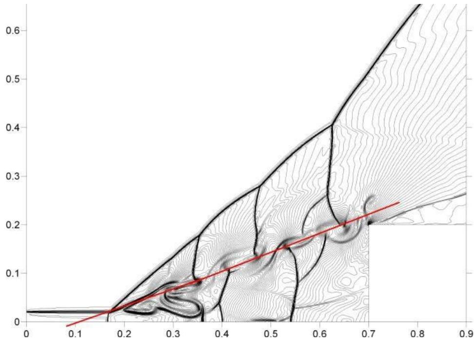
**Figure 5.** Development of Kelvin-Helmholtz shear instabilities in shock layer during interaction of heat irregularity with shock layer
