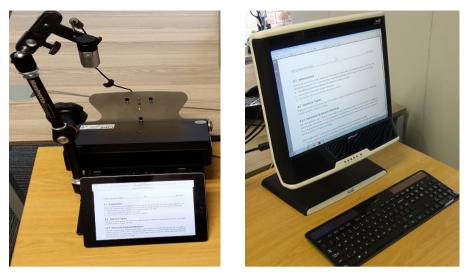
a.Tobii X120 and iPad b.Tobii T120 Eye Tracker **Figure 3.** Eye trackers – Left: Tobii X120, Right: Tobii T120 Eye Tracker
