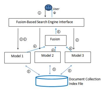
Figure 1: Structure of a fusion-based information search system
