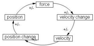
Figure 4. Feedback loop in spring mass system model
