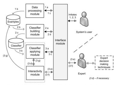
Fig. 6. Modules and main processes within the interactive classification system.
