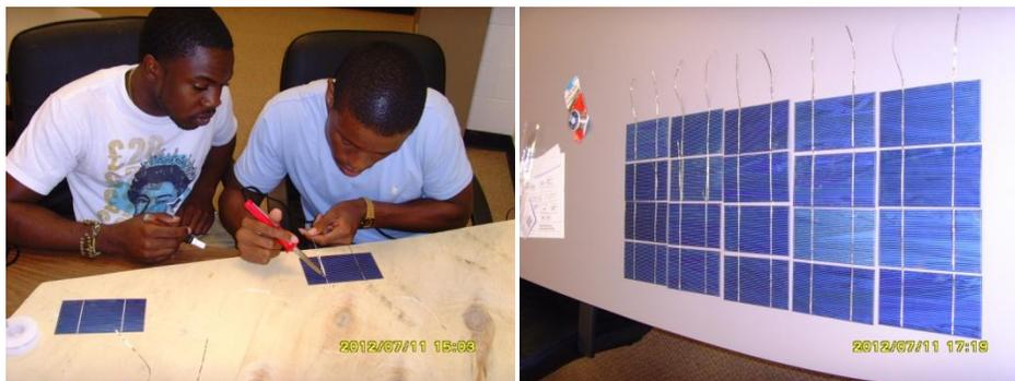
**Figure 11: Photovoltaic Panel DIY: Tabbing & Soldering**
