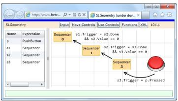
Figure 11. Propagation of triggers in the second assignment
