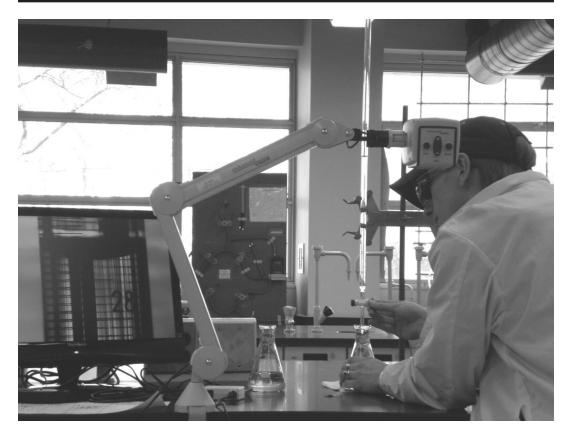
*Figure 1.* The apparatus being used in the distance view during a titration. The meniscus and the gradations of the burette are seen on the LCD screen at the left.
