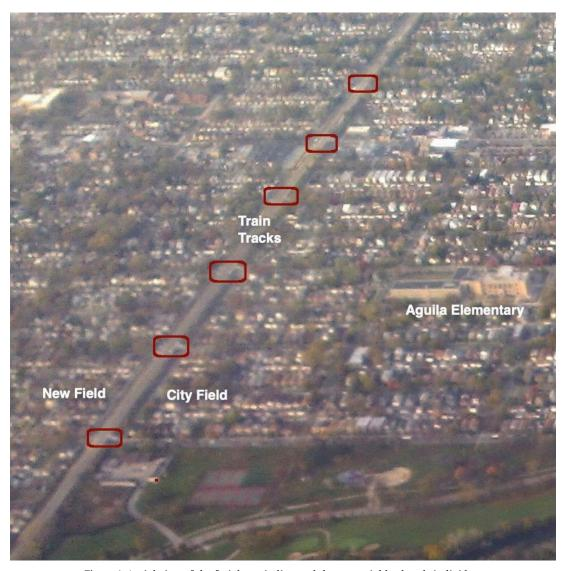
Figure 1. Aerial view of the freight train line and the two neighborhoods it divides. The viaducts, labeled in red, are located every two blocks beneath the train line tracks
