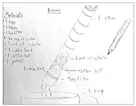
Figure 6. Cilantro filter prototype
