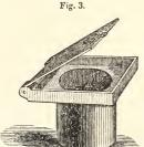
Each desk is fitted up with a glass ink-well (Fig. 2.) set firmly into the desk, and covered with a lid. The ink-well may be set into a cast iron box (Fig. 3.) having a cover; the box being let in and screwed to
