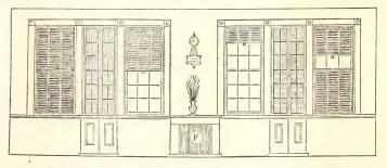
Each Schoolroom is lighted by four windows; and in the central pier, between the windows, are the Cold-air and Chimney Flues, or the Furnace Flues. The Fire-place, or Furnace Flue, is represented at F, as in the preceding Plans of the different Stories. The arrangement of the Flues, in this pier, will be seen in the next diagram.
