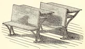
The end piece, or supports, both of the seat and desk, are cast iron, and the wood work is attached by screws. They are made for one or two scholars, and of eight sizes, giving a seat from ten inches to seventeen, and a desk at the edge next to the scholar, from seventeen to twenty-six inches from the floor.
