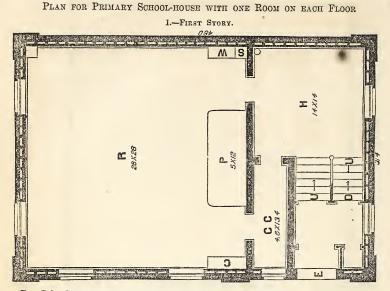
R.—School-room. P.—Platform. C.—Cabinet. H.—Hall. W.—Wardrobe with Ventilator adjoining. V.—Extra Ventilator. S.—Ventilator in connection with Sinoke Pipe.
