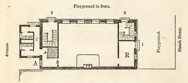
It will be seen, from this Plan, that the building was to have an end fronting on Sheafe street, (from which it was to be set back nineteen feet,) and a side looking into two of the Playgrounds, each of which was to be twentyseven by thirty feet. The nineteen feet between the building and the street, and on a line with the building, the whole extent of the fifty-three feet on Sheafe street, was to form a third Playground.
