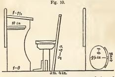
The following cut (Fig. 10) represents a range of seven desks and seats, divided by a partition (a) of matched boards, extending from the floor to three inches above Fig. 11.
