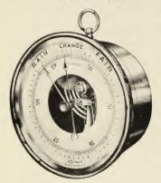
An aneroid barometer. Air pressing against a diaphragm to which is attached a spindle causes the spindle to move. The indicator attached to the spindle registers the amount of this motion on a dial. When the air pressure is increasing, the indicator moves toward the right; when the air pressure is decreasing, the indicator moves to the left. How does the indicator move when the barometer is carried in an airplane to a high altitude? To a lower altitude? above us to press down on the mercury.
