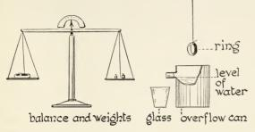
small glass to catch the water from the overflow can, and the ring to be tested.
