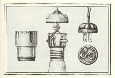
This diagram may help you to wire electric devices at home. Notice that the insulation should be torn off the ends of the wire only where they are fastened under the screws
