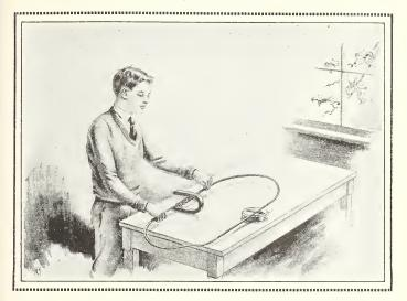
This boy, in moving the wire back and forth through the poles of the magnet, causes the magnetic needle to move
