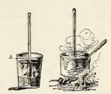
mometer plunged into melting ice. Temperature, 32°.
