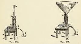
Whether there be a simple tube AD, or a large funnel, the water flows to G, 8 inches from F; for it is not the quantity of water that influences the force of the jet: it is the shot that is important.
