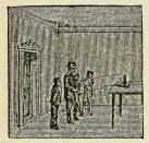
FIG. 82.—A little spark appears at each union and separation of the two wires.
