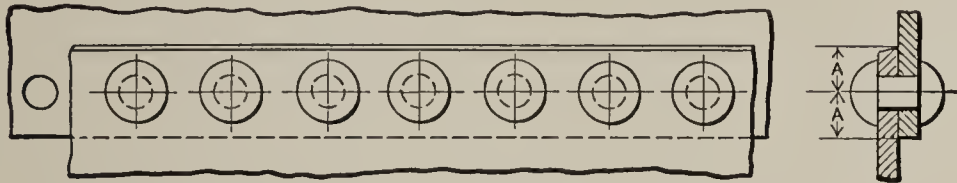
SINGLE RIVETED LAP JOINT; 1 EFFICIENCY ABOUT 56 %
