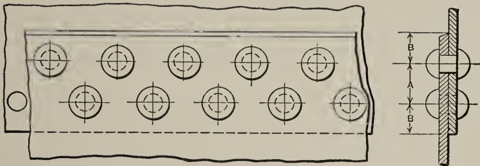
DOUBLE RIVETED LAP JOINT; EFFICIENCY ABOUT 70 %
