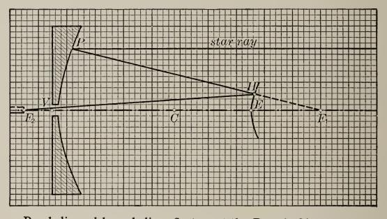
Parabolic and hyperbolic reflectors at the Detroit Observatory The curvature of the large parabolic mirror is greatly exaggerated on the diagram.
