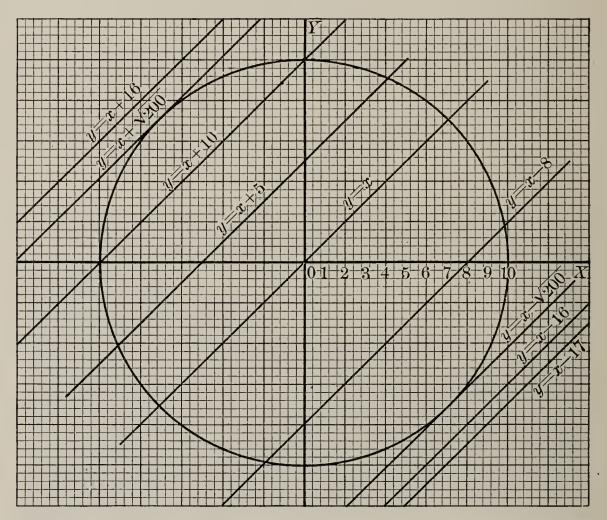
Graphical solution, determining intersections of the circle,  $x^2 + y^2 = 100$ , with various lines of slope 1
