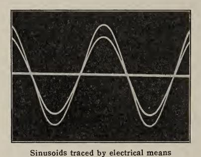
Oscillogram of an alternating current in which current and e. m. f. are " in phase." *p*, measured in watts of an ordinary electric current.
