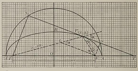
Tangent to an ellipse constructed from the focal radii to the point of tangency
