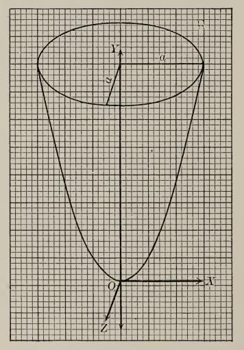
Elliptic paraboloid of revolution
