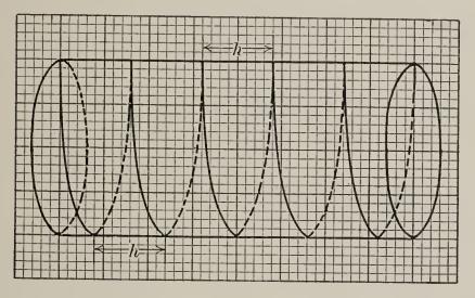
Full size representation of a one-inch cylindrical screw The '' lead '' is  $\frac{8}{20}$  of an inch.
