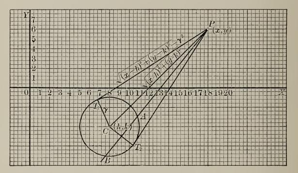
Distances from a point to a circle On any secant through P, PAB, PA × PB is constant.  $PA \times PB = \overline{PT_1}^2 = (x - h)^2 + (y - k)^2 - r^2.$
