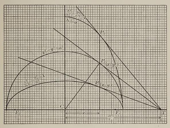
Tangent to an ellipse constructed from the tangent to the auxiliary circle a the corresponding point
