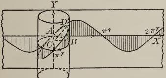
Sinusoid developed by means of a circular cylinder
