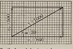
Vertical and horizontal components of a given velocity
