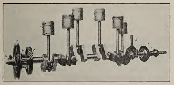
Connecting rods and crank arms in six-cylinder automobile engine: ratio l: r = 3:1
