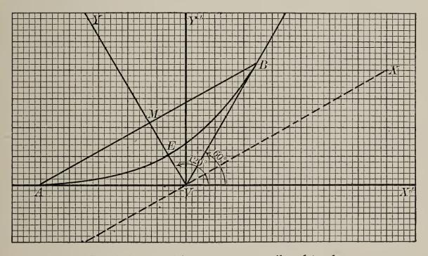
Parabolic transition curve on a railroad track The parabolic arc is used for vertical as well as for horizontal transition curves.
