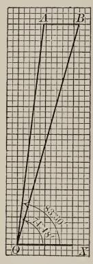
Moving aëroplane 17. In the figure AB represents the movement in 30 seconds of an aëroplane moving parallel to OX at rate of 120 miles per hour;  $\angle AOX$  is measured as 83° 30' and  $\angle BOX$  is measured as 74° 48'; find the distance OBand the position of the aëroplane at the end of the next 30 seconds if it continues on its present course.
