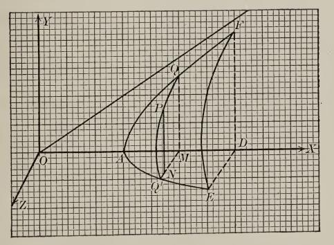
Hyperboloid of two sheets, of revolution The curves are slightly distorted.
