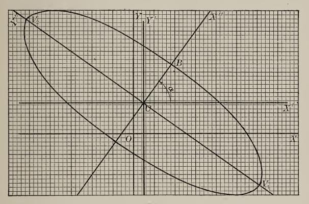
The ellipse  $3x^2 + 6xy + 5y^2 - 12x - 18y - 24 = 0$ or  $3x'^2 + 6x'y' + 5y'^2 - \frac{81}{2} = 0$ , or  $7.16x''^2 + .84y''^2 = 40.5$
