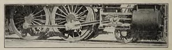
Connecting rod, crank arm, and cylinder on A. T. & S. F. locomotive 1444. The stroke is 30 inches and connecting rod 60 inches.
