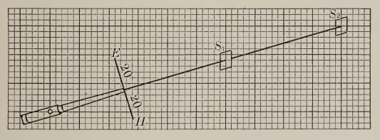
Distances of screens from muzzle, *M*, determined by right triangles Two screens spaced 100 feet apart (horizontally).
