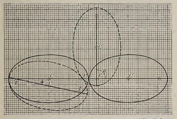
Two positions of elliptical gears, mounted on corresponding foci Note that the right-hand ellipse swings through a large angle, in this position, as compared with the left-hand one.
