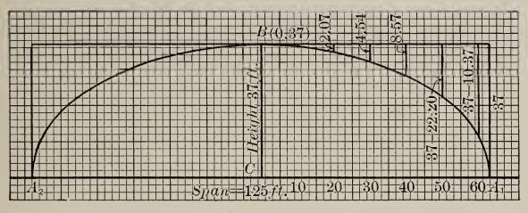
Elliptical arch, 125 foot span by 37 feet high
