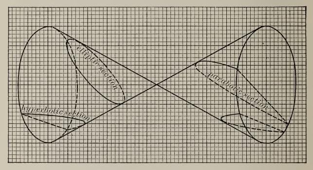
Ellipse, parabola, hyperbola, and two straight lines as intersections of a cone by a plane
