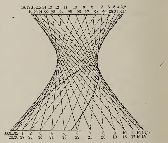
The right-line generators on this hyperboloid of revolution are formed by connecting corresponding points on two circular sections An elliptic section is also indicated.
