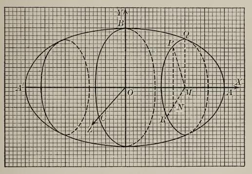
Ellipsoid of revolution, with x-axis as axis of revolution
