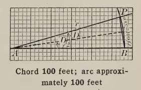
subtended by a chord whose length is 100 feet, the length of one chain used in surveying. On a simple curve the lengths
