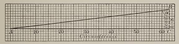
Circumference, AC, and length of one spiral, AB, of the above one-inch cylindrical screw
