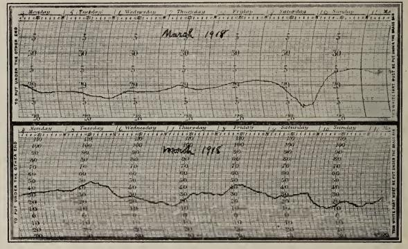
Temperature and barometric chart by moving pointer
