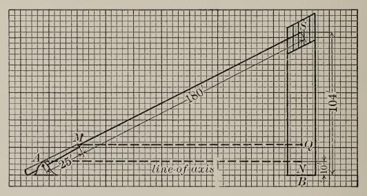
**Determination of velocity** of a projectile One screen is at the muzzl of the gun.
