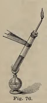
The gas once lighted causes a flame, whose heat melts the wax below; and the liquid, lifted by capillary force through the wick, is changed to vapor as fast as it is needed in the flame. Take the wax in a test-tube with a jet-pipe through its tight cork, and heat it. The wax melts, then boils, and the vapor at length issues from the jet, when, if touched with a lighted match, it burns (Fig. 76) with exactly the same kind of flame, only less steady.
