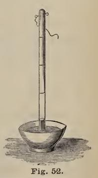
The Experiment. — The apparatus consists of a eudiometer, shown in Fig. 52. Four equal divisions are marked off from the closed end of the tube. Two of these divisions are filled with nitrous oxide; the remaining two are afterward filled with pure hydrogen. By an electric spark a violent explosion is made; steam is condensed on the side of the tube, and water from the cistern will rise, leaving the two upper divisions only filled with gas. This gas, when tested, is found to be nitrogen.
