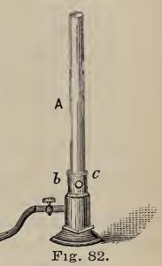
The instrument is much used in the  $F_{1g. 82.}$ laboratory for heating glass vessels,  $F_{1g. 82.}$ for which it is well adapted, because its flame is without smoke and deposits no soot.
