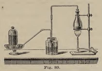
there is a *flask*, in which the organic matter is heated; a *bottle* surrounded by cold water, in which impurities are condensed; and a *receiver* over water, in which the gas is collected. These three parts of the apparatus are represented in every
