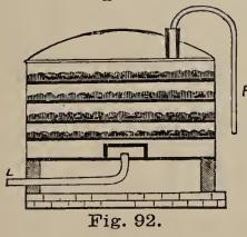
ing sulphur compounds and carbonic acid, passes from the condensers through a pipe (L) into a chamber (Fig. 92) in which are several sievelike shelves covered with slaked lime. In passing through the lime the gas loses its carbon dioxide and hydrosulphuric acid.
