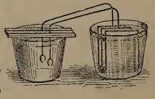
of the former metal, with a strip of copper fastened between the two portions. The Explain the figure. metals should be within an eighth of an inch of each other, but without contact. To secure this, they are tied together with thread, bits of wood or cotton cloth being previously interposed. Copper wires being attached to the zinc and copper, as represented in the figure, the apparatus is placed in a common tumbler, and the battery is complete.
