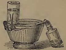
bowl, and let the remaining water run out. The air will immediately rush in and change the colorless nitric oxide to red vapors of the peroxide of nitrogen.
