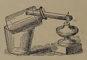
into a vial or flask. It is necessary to keep the vial covered with porous paper or cloth, and to moisten it frequently in order to maintain its coolness. Where larger quantities are prepared, a retort and well-cooled receiver are employed, as represented in the Appendix.
