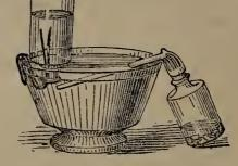
as represented in the figure. The evolution of the gas immediately commences. The first portions, which contain an admixture of air, are allowed to escape; the pipe-stem is then brought under the mouth of the vial, and the gas collected.\*
