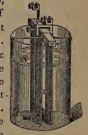
from one-seventh to one-sixteenth of its bulk of oil of vitriol, is employed in this battery. It is generally used in plating.
