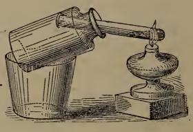
A little sand may be added to the mixture with advantage. The vial should be kept cool by means of paper repeatedly moistened during the process. The space between the tube and the neck of the vial should also be loosely closed with wet paper.
