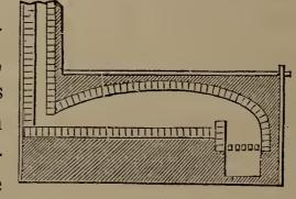
of soda, chalk, and coal, are heated together in a reverberatory furnace, the carbonate of soda is then dissolved out from the fused mass, dried, purified, and subsequently crystallized. The sulphide of calcium would dissolve at the same time, and thus defeat the process, were it not rendered insoluble by combination with a certain quantity of lime.
