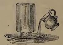
the cavity. Water must be poured into the saucer as the first portion rises into the bottle. The bottle is then cooled, either by water or long standing, and corked while yet inverted It is then shaken, to wash the gas. A piece of phosphorus, of the size of a large pea, is sufficient for the preparation of half a pint of gas.
