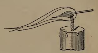
The oxide to be reduced, is to be placed within the yellow body of the flame, but near its termination. The litharge produced in the last experiment, may be re-converted, by this means, into metallic lead.
