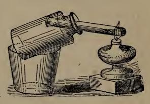
cing the mouth of the test-tube, containing the proper materials, in a wide-mouthed vial, and heating, as before. As the gas is evolved, it will expel the air, and soon fill the vial.
