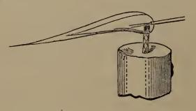
which, within its fainter blue envelop, the metal is to be held. A piece of lead, of the size of a grain of wheat, placed on charcoal, hollowed out for the purpose, and exposed to the flame, will soon be converted into litharge. The oxide will be recognized by the yellow incrustation which it forms upon the charcoal support
