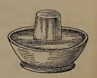
ting gas, from public gas works, is effected on the same principle. The weight of the sinking gasometer, is sufficient to press it through pipes, to all parts of a large city.
