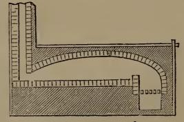
the constant stirring which is essential, such a furnace for refining iron is called a puddling furnace. The
