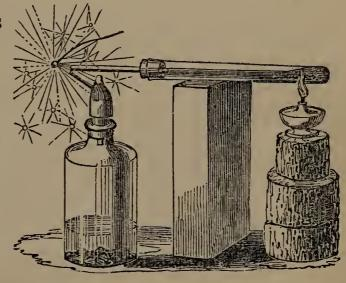
by galvanic means. Iron, copper, zinc, and other metals, melt and burn in it readily; the former, with beautiful scintillations, and the latter, with characteristic colored flames. With a sufficiently constant flame
