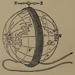
net. A freely movable coil through which a current was passing, would, in this case also, act precisely like a magnet.
