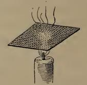
holding down a piece of wire gauze upon the flame of a candle. If the gauze is fine, the flame will not pass through it. This effect is owing to the reduction of temperature which the wire occasions. The subject will be better understood by reference to the paragraphs which follow, on the nature of flame.
