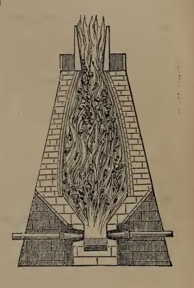
become more thoroughly heated, and meet carbonic oxide from the coal below, which robs the iron of its oxygen, and converts it into particles of metal. Still lower down, the lime combines with the earthy portions of the ore, forming a liquid glass. The reduced iron thus liberated, collects, fuses, and sinks to the bottom of the furnace. From this point it is run off into channels of sand, where it hardens into pig iron.
