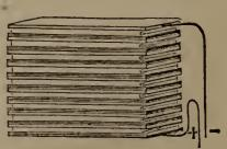
lations of the burning metal may also be readily produced. By increasing the number of the plates still more striking effects are obtained. With a pile consisting of six or eight plates a foot square, platinum wire connecting the electrodes may be readily fused. Such a battery is also more effectual in the electromagnetic experiments which follow.
