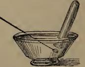
in the figure. The metal melts as soon as it touches the water, and rises to the top of the tube. Hydrogen is immediately formed, and displaces the water, filling the tube rapidly with the liberated gas.
