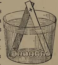
with the next chlorine, the hydrogen of this, with the next, and so on, as before explained, in the decomposition of water. Hydrogen is therefore constantly given off at the surface of the copper. But when the two metals are not in contact above the liquid, and the circuit is, consequently, not completed, there is no negative influence exerted at the extremity of the copper, and the series of decompositions, before described, does not occur.
