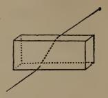
28. The figure represents a block of glass, and shows the direction which a ray of light would take on entering and emerging from it. On entering, it makes a bend, and passes on through the glass less obliquely; that is, more nearly in the direction of a line drawn perpendicularly to the surface of the glass, and continued through it. On passing out again it would be bent away from such an imaginary perpendicular line, and re-assume its previous course.
