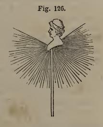
rise and repel each other. A toy is in this way constructed, representing a person under excessive fright. On touching the head with the hand, or any conducting substance, not insulated, the hair will fall.
