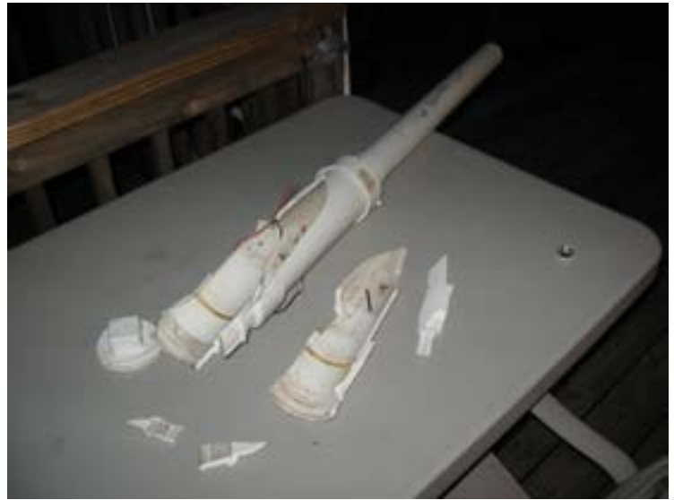
A potato gun that exploded.
