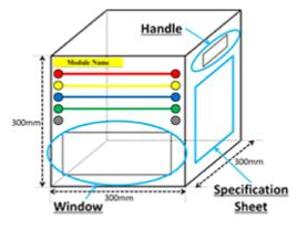
Figure 1. Standard of Module-Type Power System Training Device
