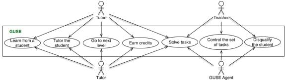
Figure 1. Use case diagram for the GUSE.
