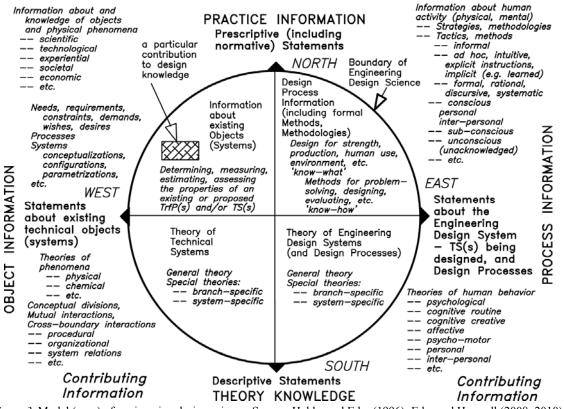
Figure 3. Model (map) of engineering design science. Source: Hubka and Eder (1996); Eder and Hosnedl (2008; 2010).
