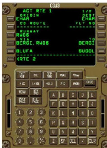
Figure 3. The simulation of a Flight Management System (FMS).
