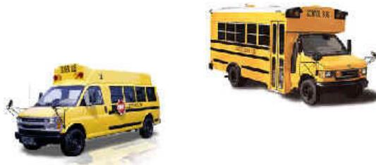
A Type “B” school bus is constructed utilizing a stripped van or truck chassis. The entrance door is behind the front wheels. This definition includes two classifications:
