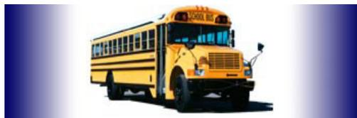
Type “D” or transit school bus is constructed utilizing a stripped bus chassis. The entrance door is ahead of the front wheels.
