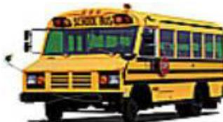
Type “C” or conventional school bus is constructed utilizing a bus chassis with a hood and front fender assembly. The entrance door is behind the front wheels.
