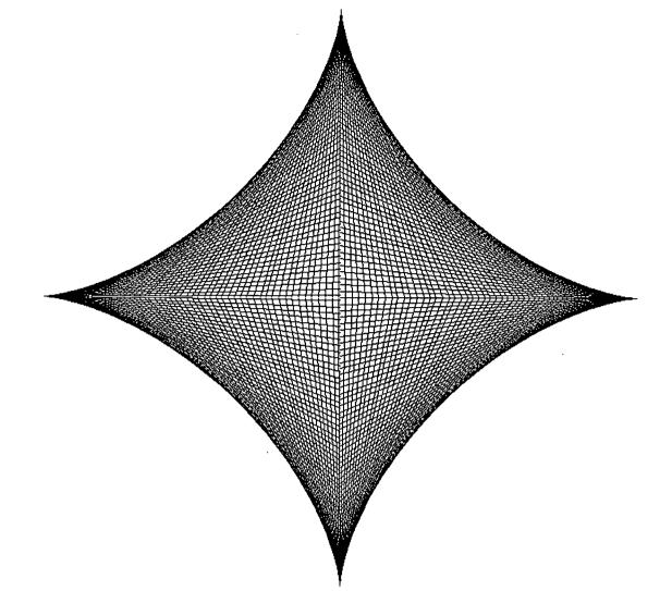
In this case all segments have the same length and have endpoints lying on two mutually perpendicular lines. The same envelop may appear as a curve touching a family of ellipses:
