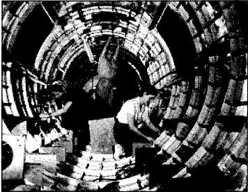
Women workers install fixtures and assemblies to a tail fuselage section of a B-17F bomber at the Long Beach, Calif., plant of Douglas Aircraft Company.
