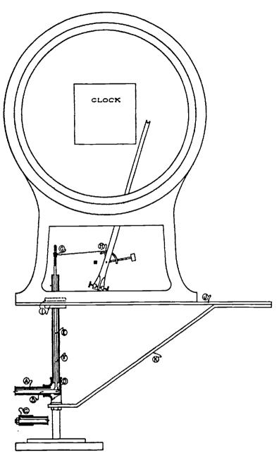
$\mbox{\bf Fig. i.}$  Showing construction of new metal thermometer and attachment to recording apparatus.
