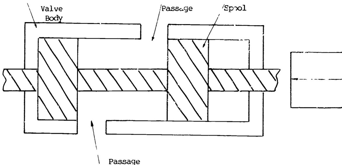
Figure 23 - Two-Way Valve (Open)
