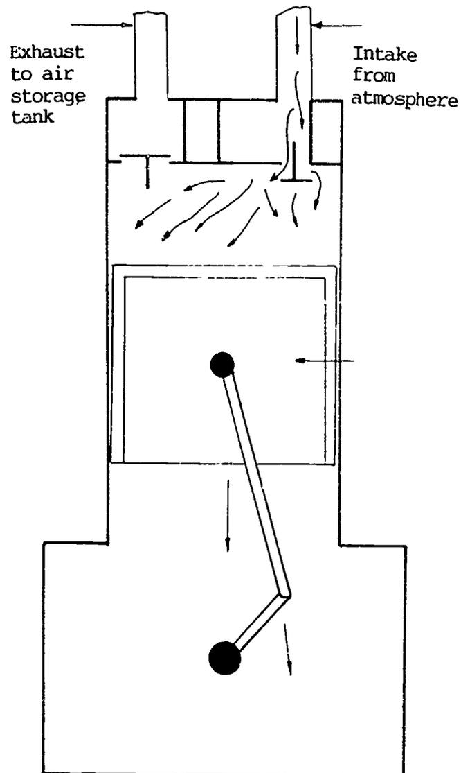
Figure 2 - Compressor, Intake Stroke
