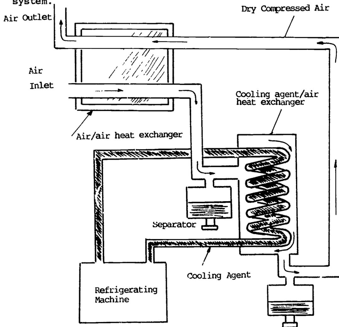
Figure 13 - Low-temperature Drier
