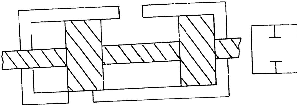
Figure 24 - Two-way valve (closed)
