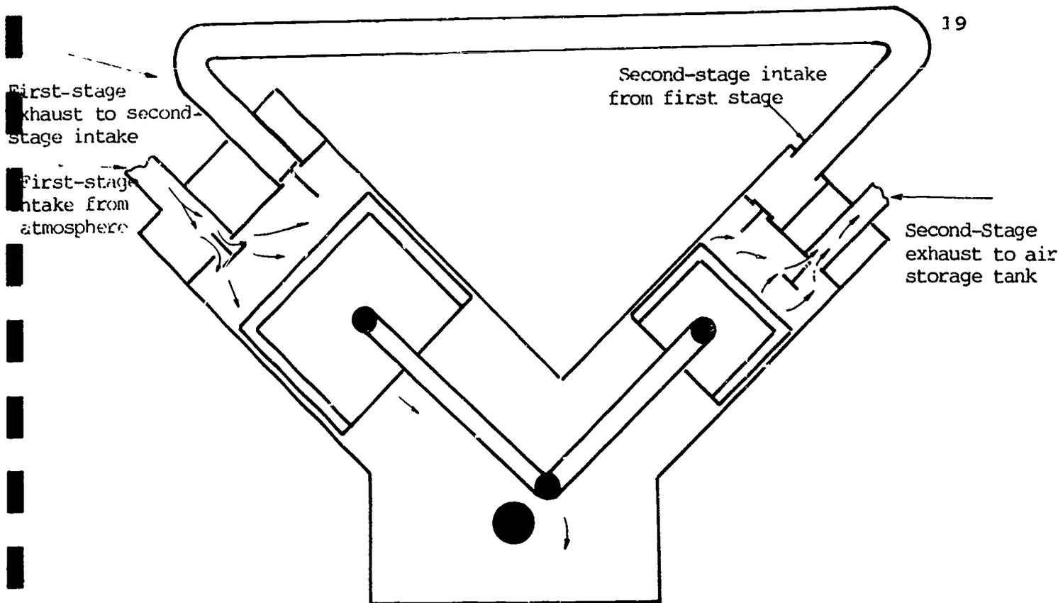
Figure 8 - Two-Stage Compressor
