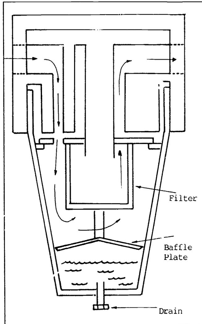
Figure 14 - Manual drain air filter
