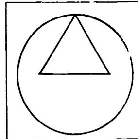
Fig. 1 Compressor Logic Symbol
