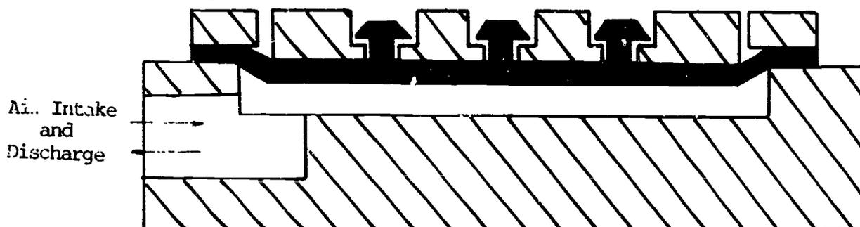
Figure 33 - Diaphragm Cylinder
