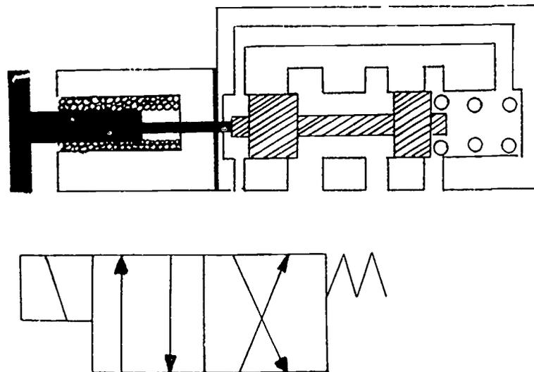
Figure 30 - Solenoid Activated Valve
