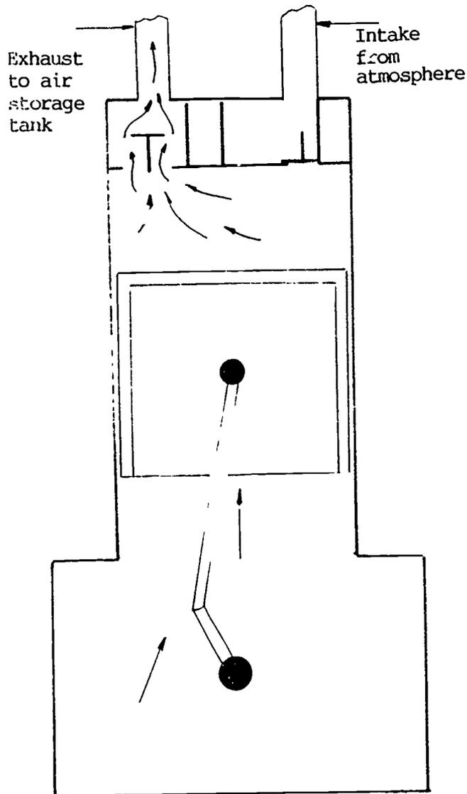
Figure 3 - Compressor, Exhaust Stroke
