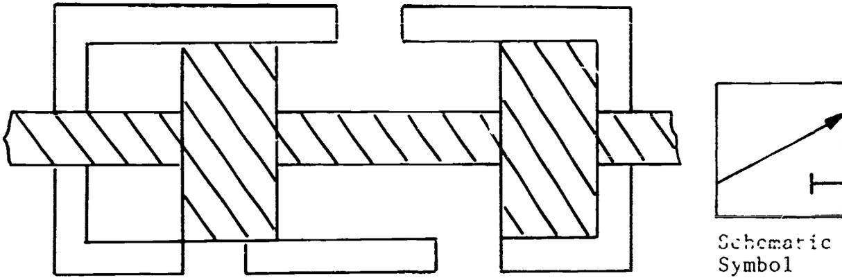
Figure 26 - 3-Way Valve - Exhaust Position
