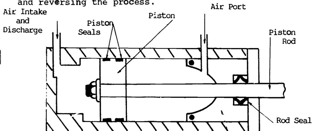
Figure 35 - Double-Acting Cylinder
