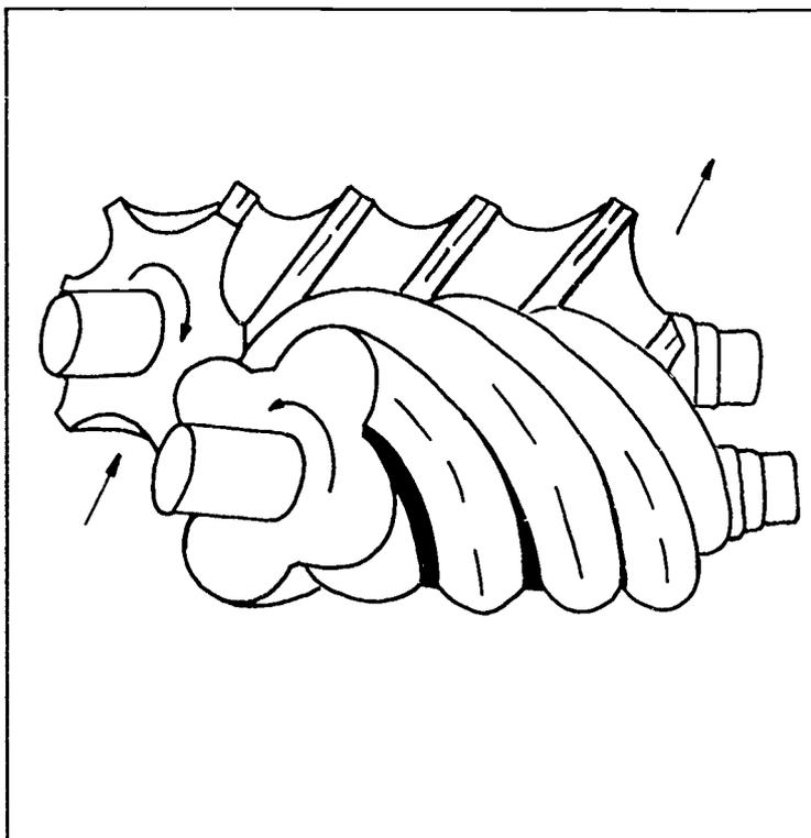
Helical compressors operate by running two meshed rotors together to generate compressed air by drawing air in one end of the compressor and exiting it from the other end. There are two basic types of helical compressors, dry or oil flooded. Both types may deliver up to 125 PSI.
