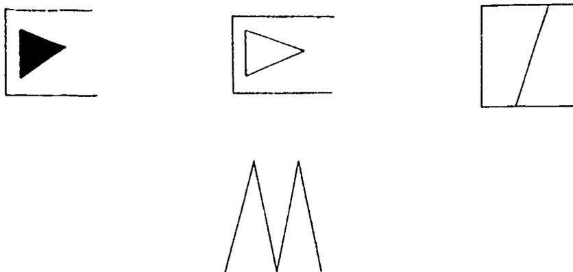
Figure 29 - Automatically Operated Valve Symbols
