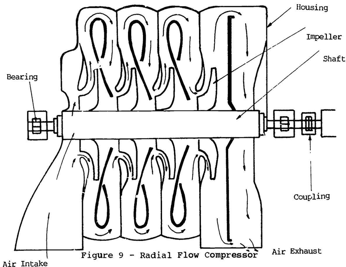
Figure 9 - Radial Flow Compressor
