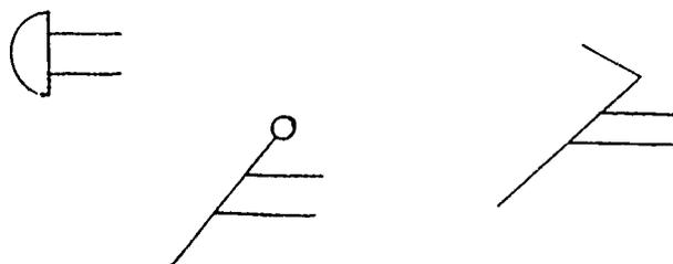
Figure 28 - Manually Operated Valve Symbols
