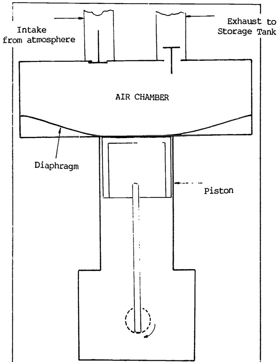
The compressor first lifts the diaphragm to draw air into the compressor chamber. As the diaphragm plate reverses its stroke, the intake valve is closed and the exhaust valve is opened. The volume of the air is reduced, and the air is piped into the storage tank. As the piston moves downward, the diaphragm also moves downward, thus increasing the volume in the air chamber. These compressors have many light duty applications, and operate at roughly 30 to 40 PSIG.
