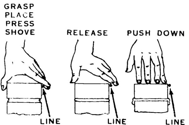
Figure 27. Laying Brick to the Line
