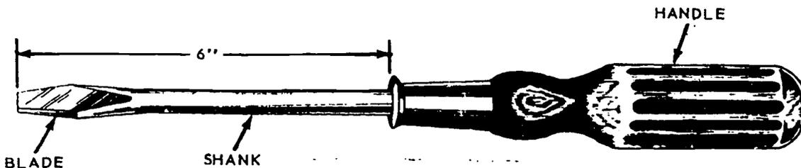
FIGURE 65. Six-Inch Common Screwdriver
