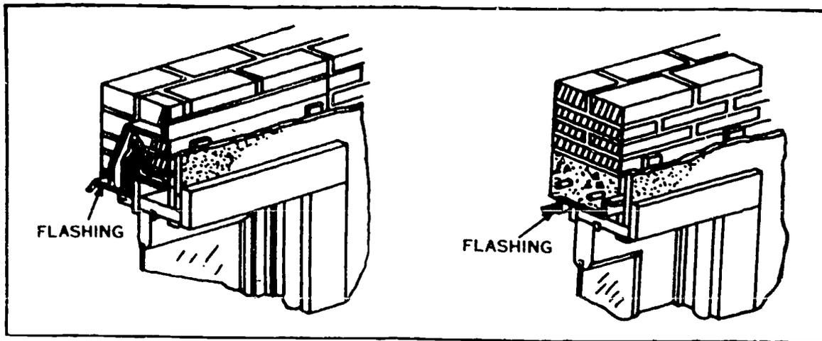
Figure 15. Head Flashings
