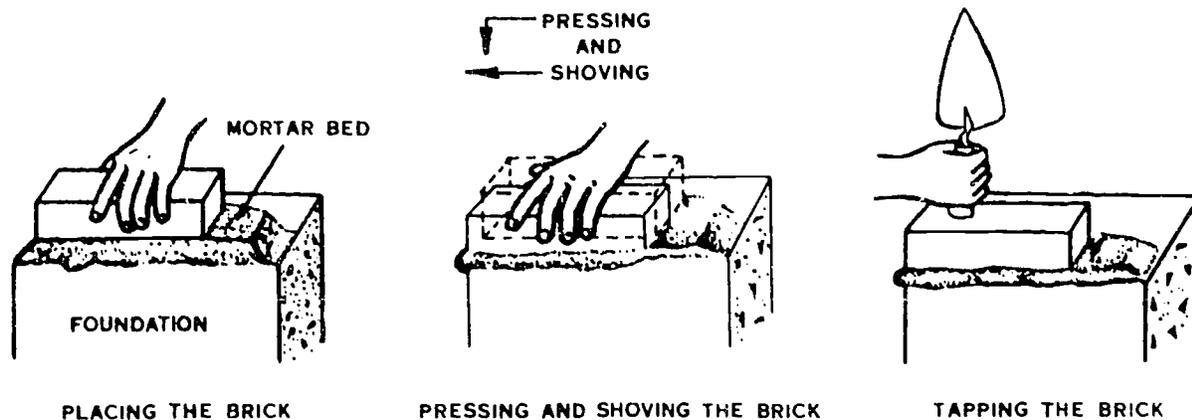
Figure 21. Positioning the Corner Brick
