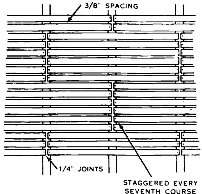
Figure 7. Proper Spacing for Wood Lath
