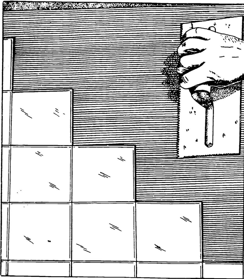
Figure 44. Spreading Adhesive with a Notched Trowel
