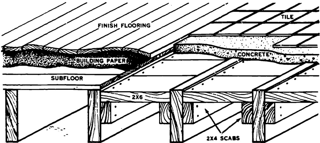
Figure 50. Recessed Concrete Base
