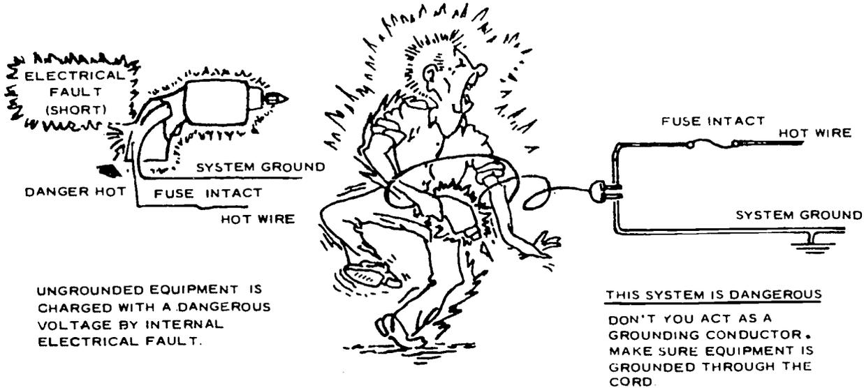
FIGURE 37. Equipment Grounding
