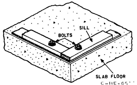
FIGURE 107. Anchor Bolts Which Are Set In Place Before Concreting
