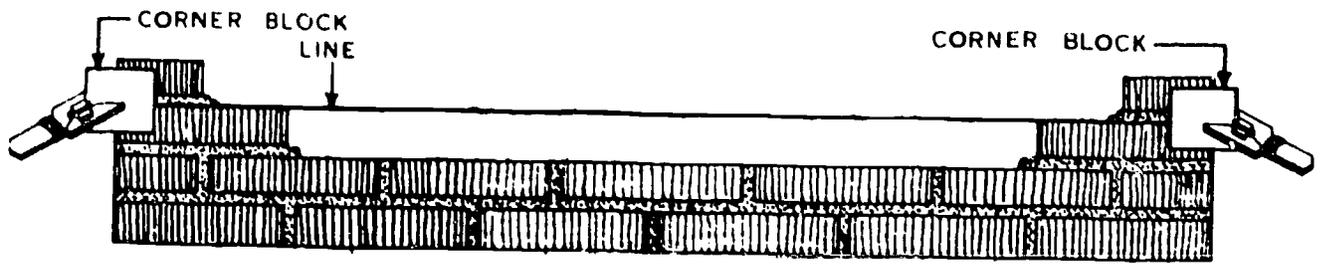
Figure 25. Line Fastened Between Corner Blocks
