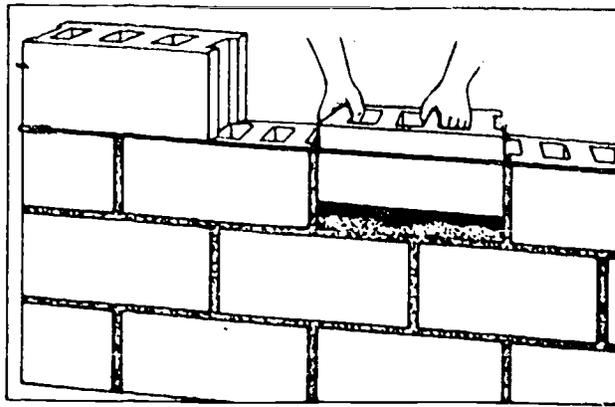
Figure 7. Laying a Closure Block to the Line
