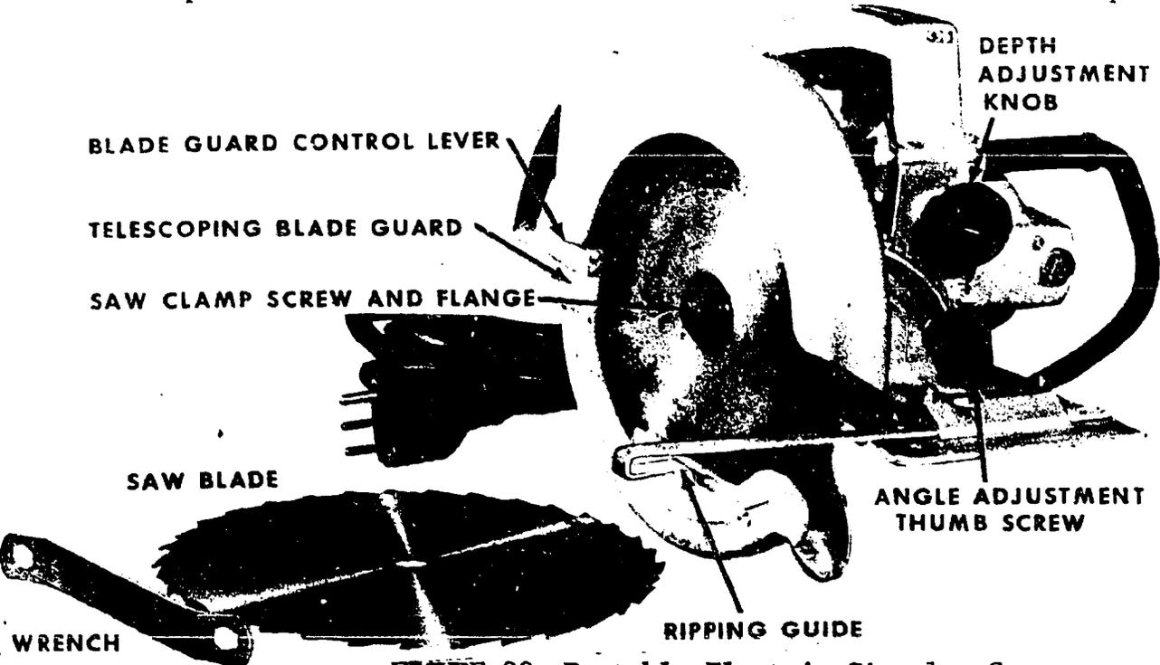
FIGURE 90. Portable Electric Circular Saw
