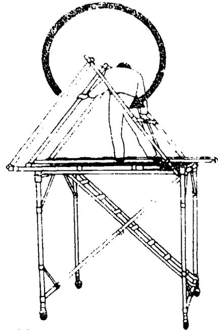
FIGURE 22. Swing the top end frame through 270°
