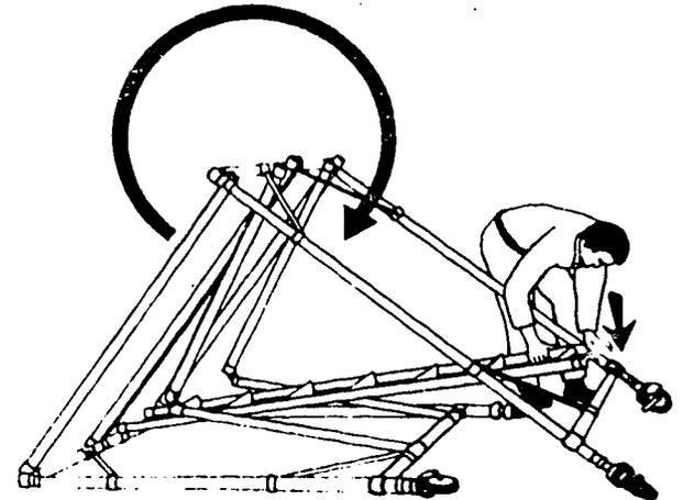
FIGURE 15. Snap the lower crossbar into the stairway hooks
