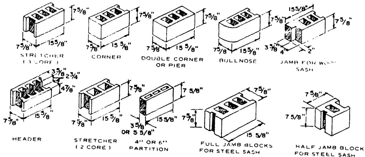
Figure 1. Sizes of Concrete Block
