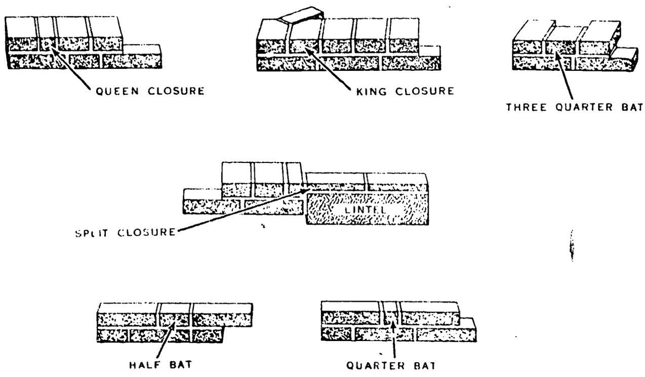
Figure 8. Various Cuts of Brick
