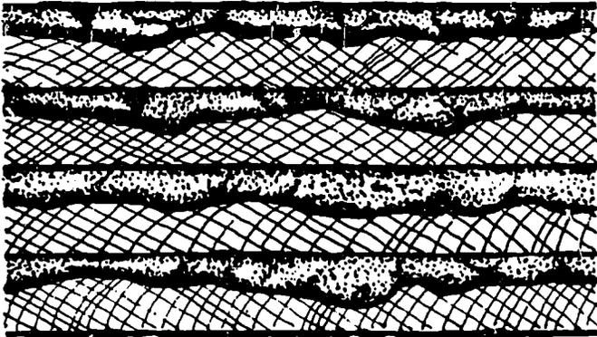
Figure 6. Wood Lath with Proper Keys
