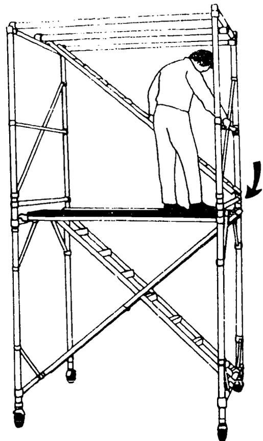
FIGURE 24. Lock the stairways hooks
