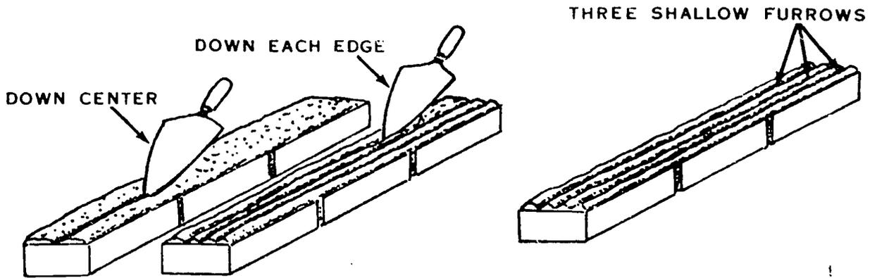
Figure 19. Riffling the Mortar
