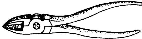
FIGURE 78. Diagonal Cutting Pliers
