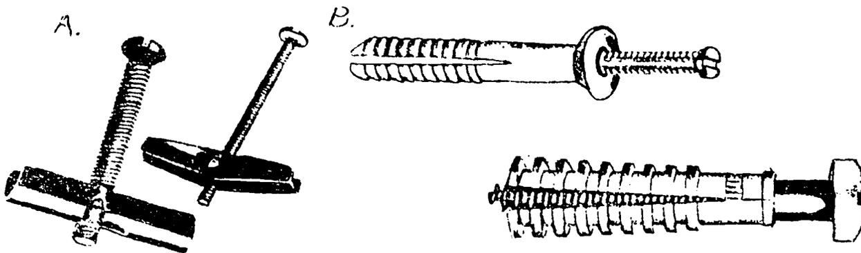
FIGURE 106. A. Shows Typical Toggle Bolts
