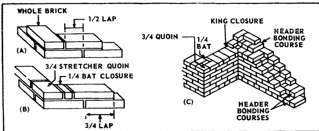
Figure 10. How To Correctly Bond A Brick Wall
