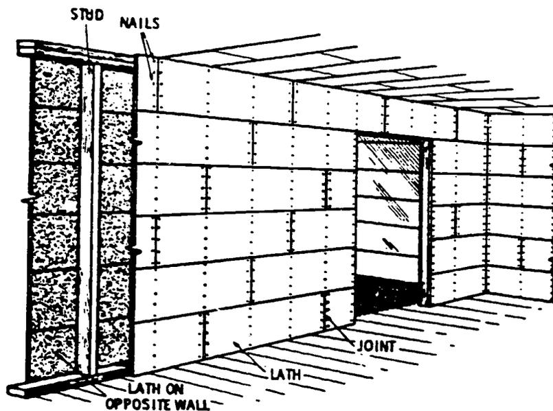
Figure 14. Gypsum Board Lath Installation
