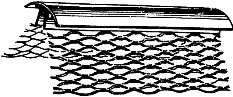
Figure 12. Bullnose Corner Bead
