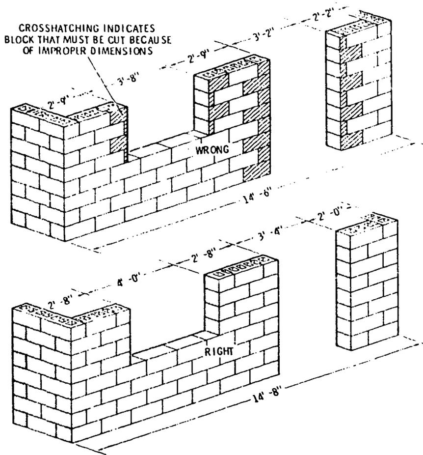
Figure 4. Proper Modular Designing
