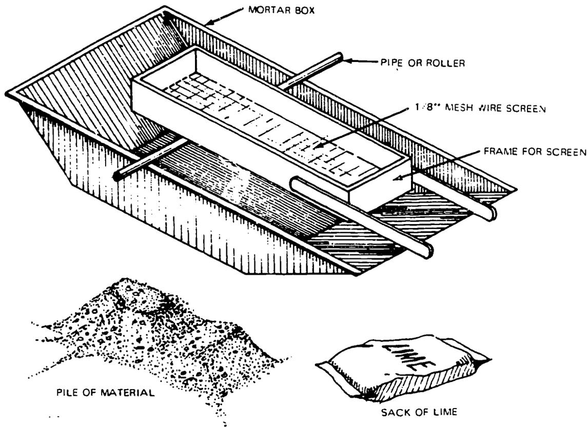
Figure 22. Mortar Box and Screen
