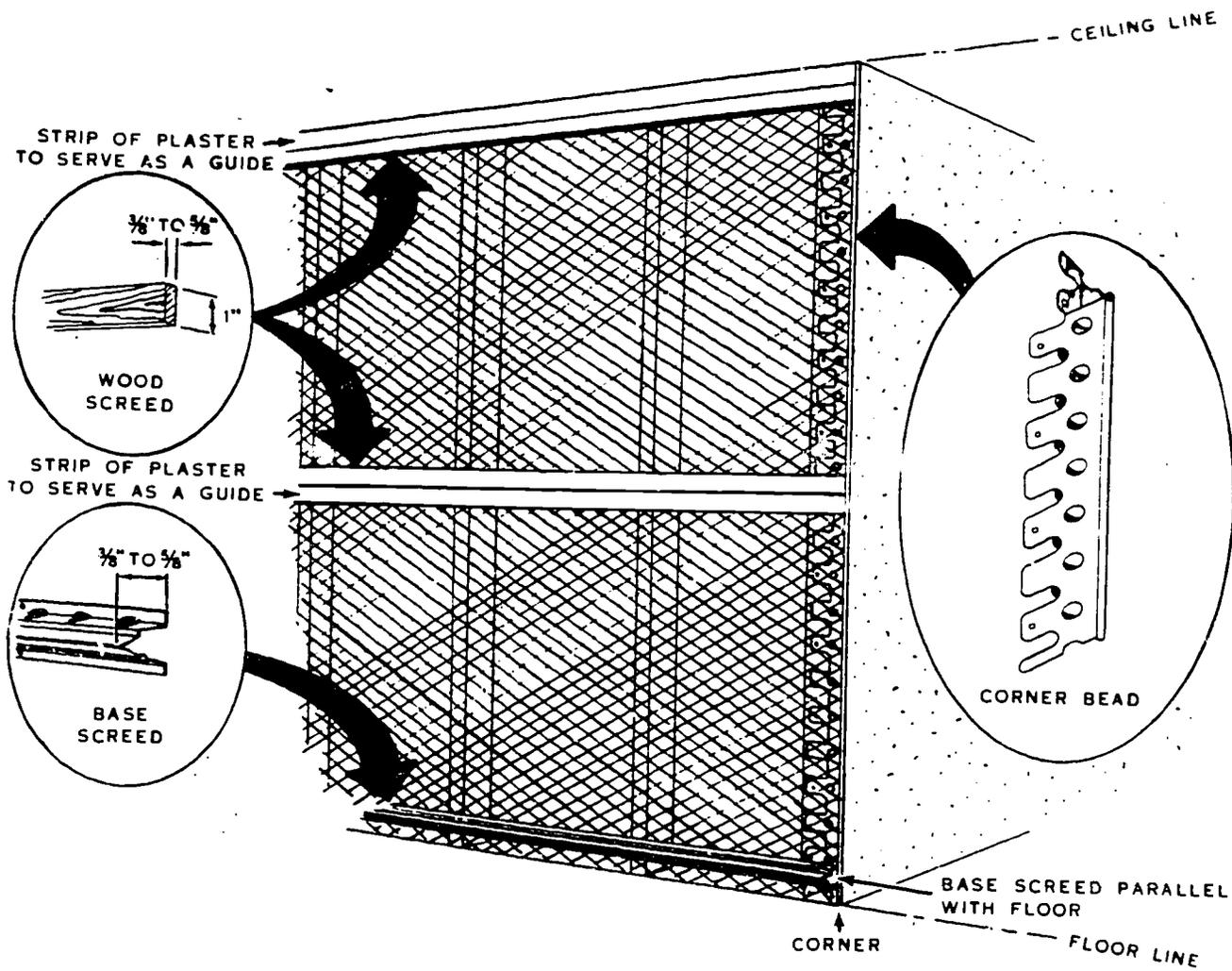
Figure 15. Placement of Screeds on a Wall
