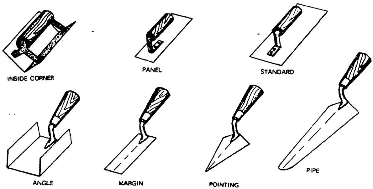
Figure 17. Types of Trowels Used in Plastering
