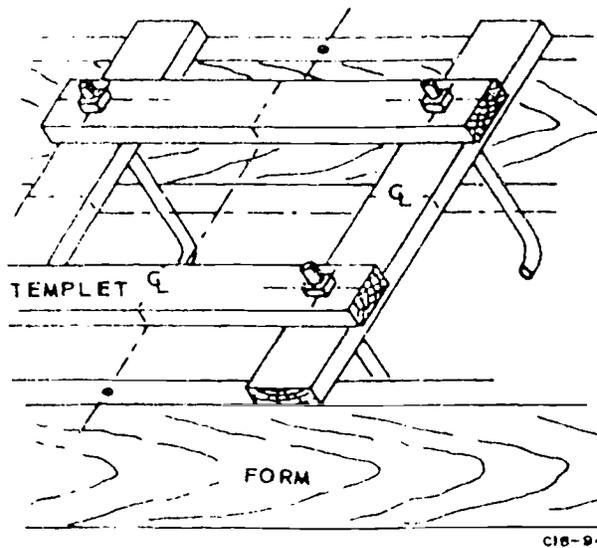
FIGURE 109. Templet for Anchor Bolts
