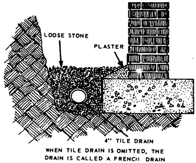
Figure 33. Tile Drain Method
