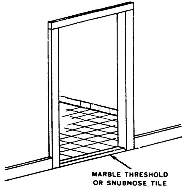
Figure 52. Finishing Doorway with a Saddle
