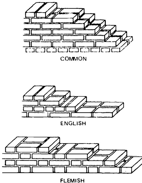
Figure 11. Bonds Normally Used for 8 Inch Walls
