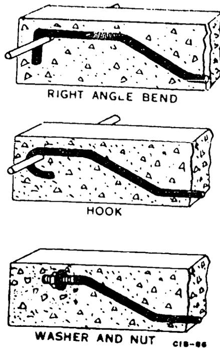
FIGURE 105. Types of Anchorage
