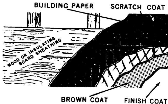
Figure 23. Three Coat Application
