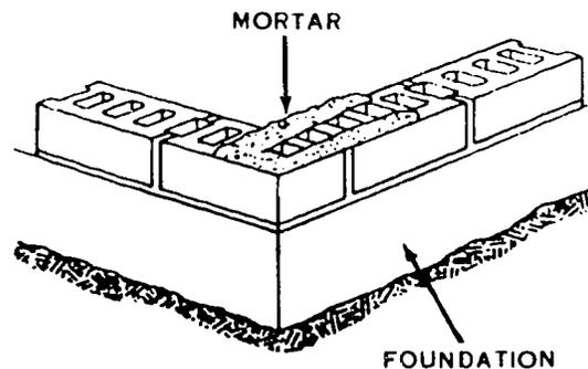
Figure 5. Mortar Swiped onto the Block
