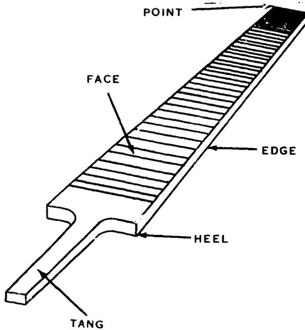
FIGURE 69. Parts of a File
