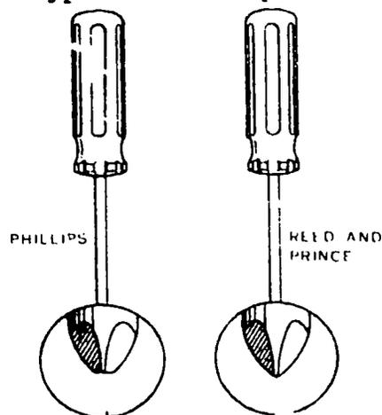
FIGURE 68. Cross-point screwdrivers
