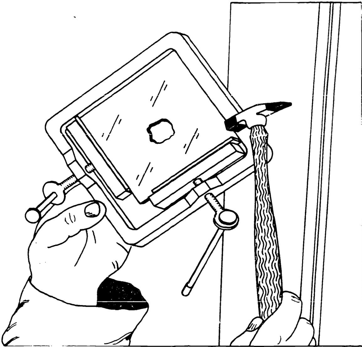
Figure 37. Making a Hole with a Hole Breaker and Tile Hammer
