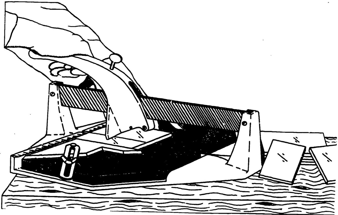
Figure 40. Breaking the Tile on a Tile Cutter
