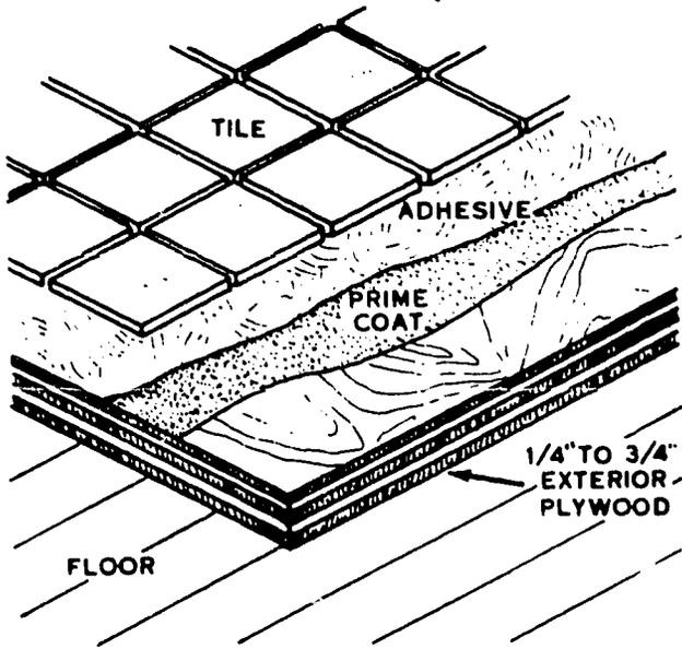
Figure 51. Preparing an Existing Floor for Floor Tile
