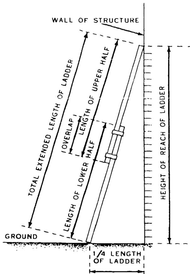
FIGURE 31. A Properly Placed Ladder
