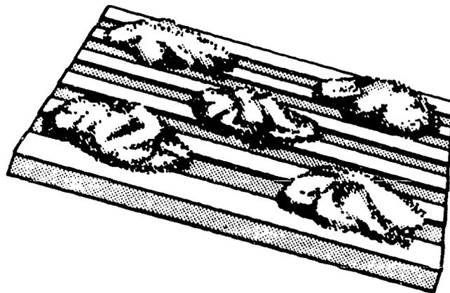
Figure 55. Buttering Quarry Tile
