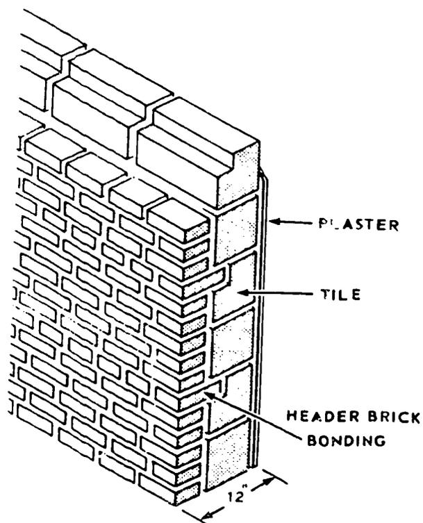
Figure 3. How Structural Tile Are Used
