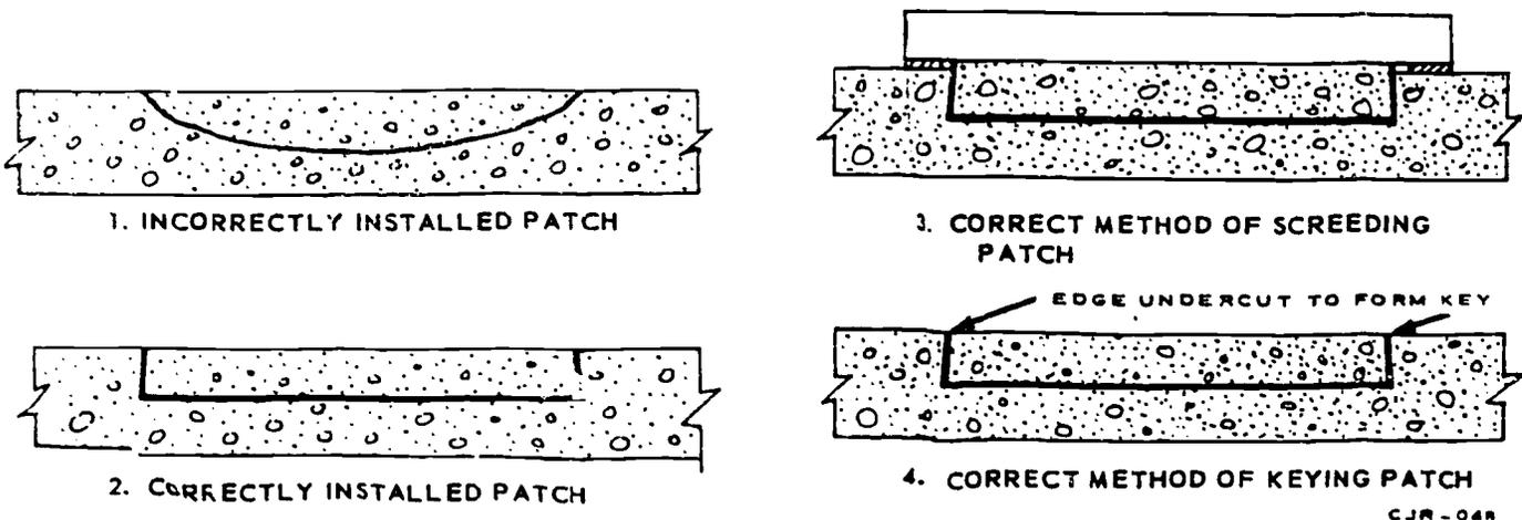
FIGURE 110. Patching a Concrete Slab
