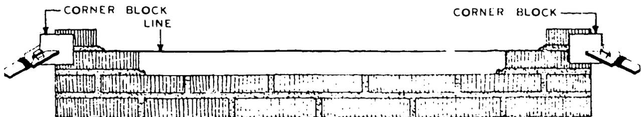
FIGURE 60. Line and Line Holders
