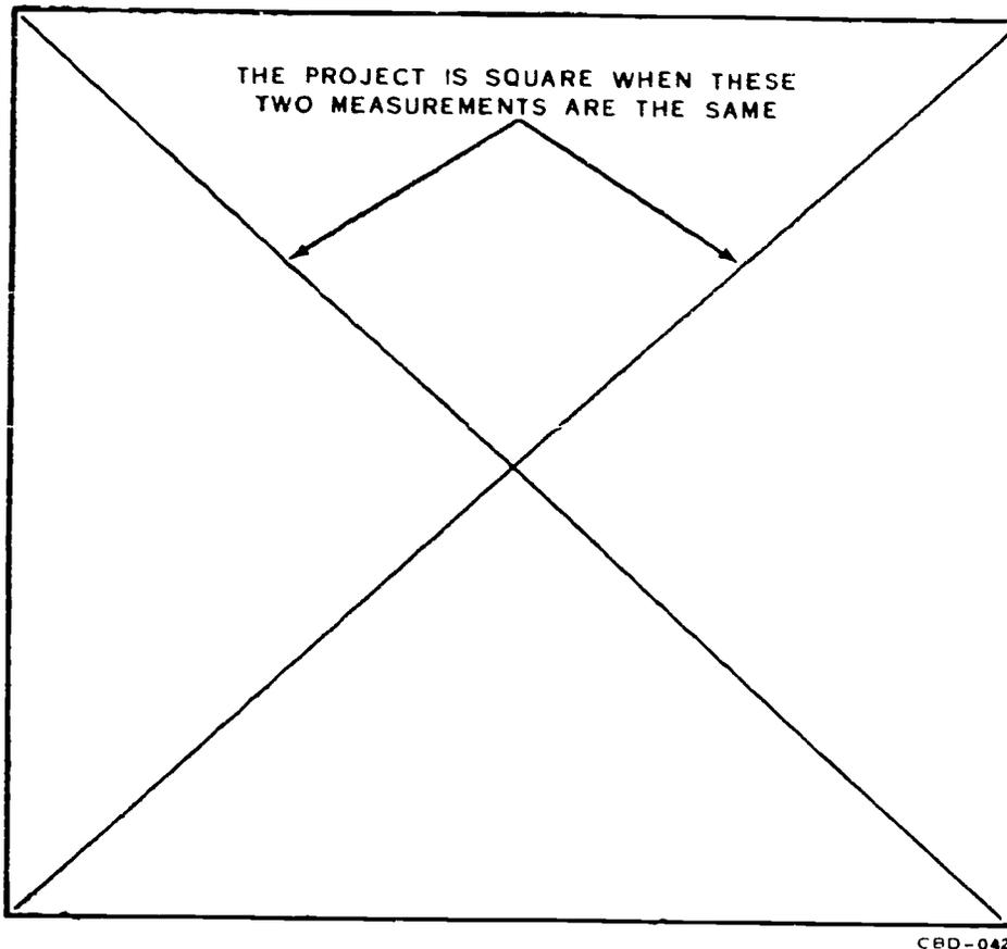
FIGURE 98. Diagonal Checking
