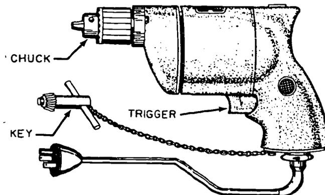
FIGURE 94. Electric Drill
