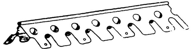
Figure 13. Standard Corner Bead
