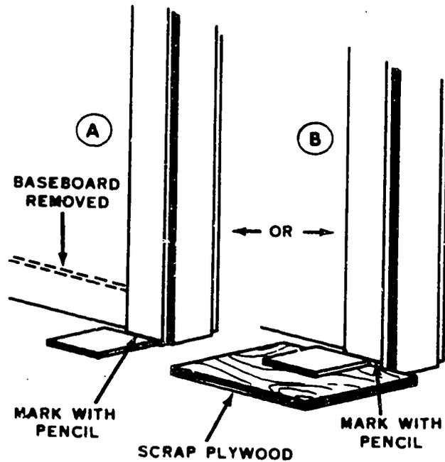
Figure 53. Marking Door Casing
