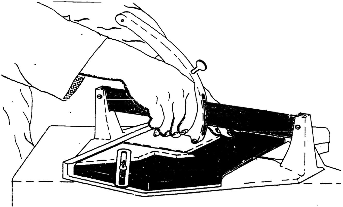
Figure 39. Scoring the Tile on a Tile Cutter
