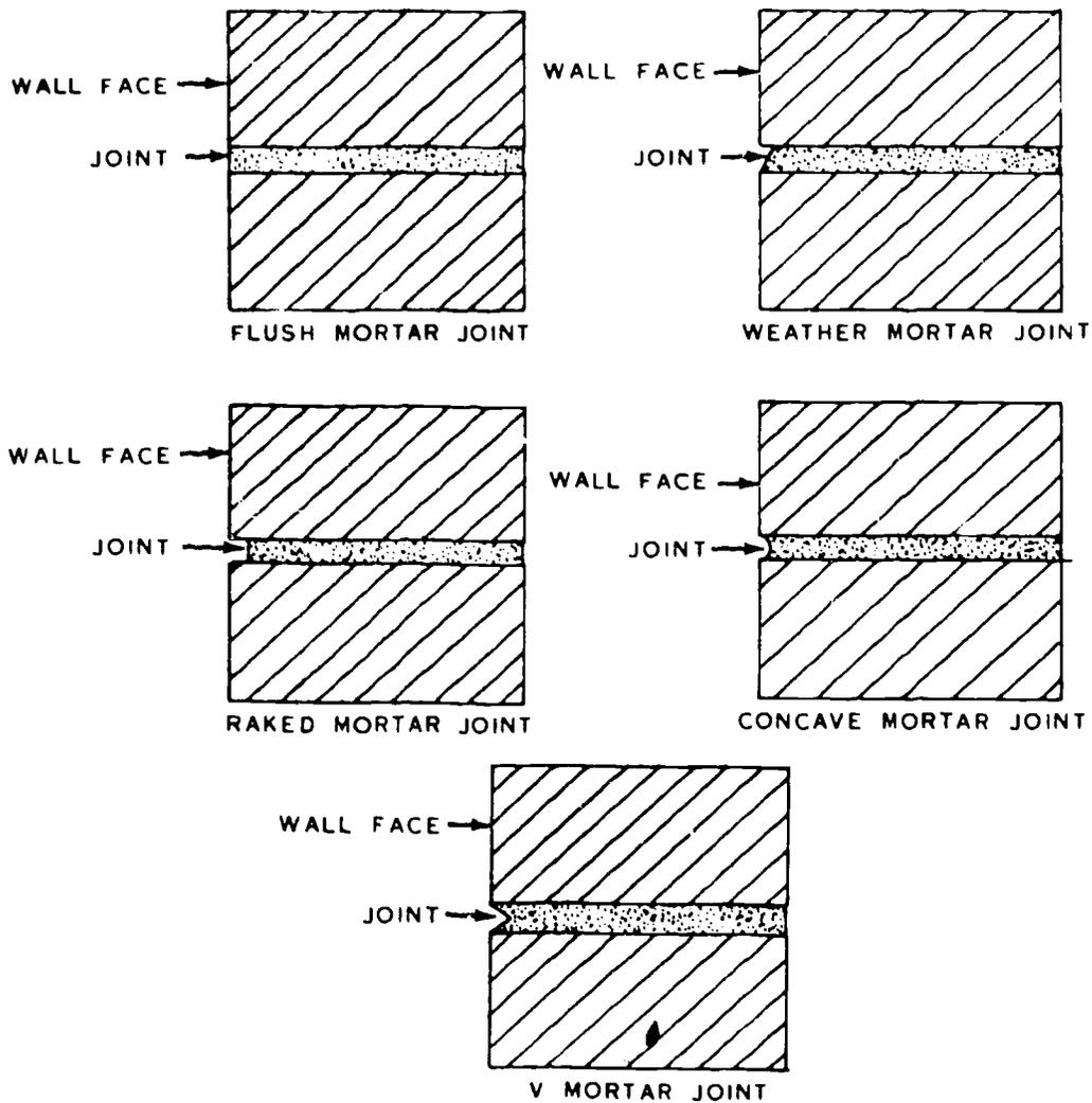
Figure 29. Types of Mortar Joints
