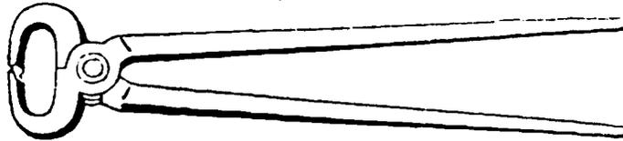
FIGURE 80. Tile Nipper Pliers
