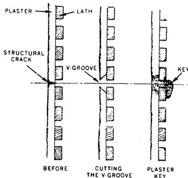
Figure 31. Repairing a Structural Crack
