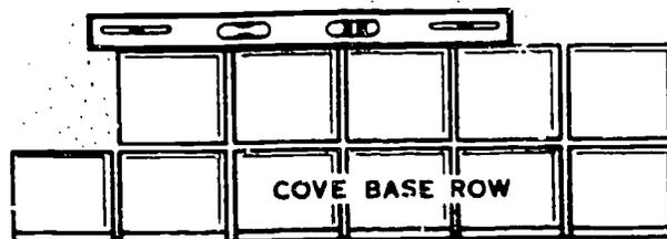
Figure 46. Leveling Wall Tile
