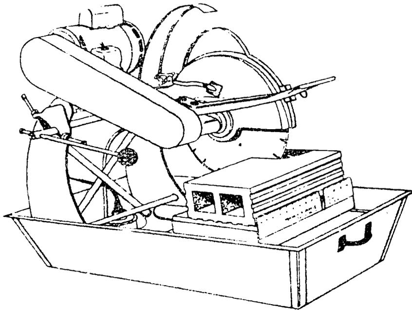
FIGURE 87. Masonry Saw
