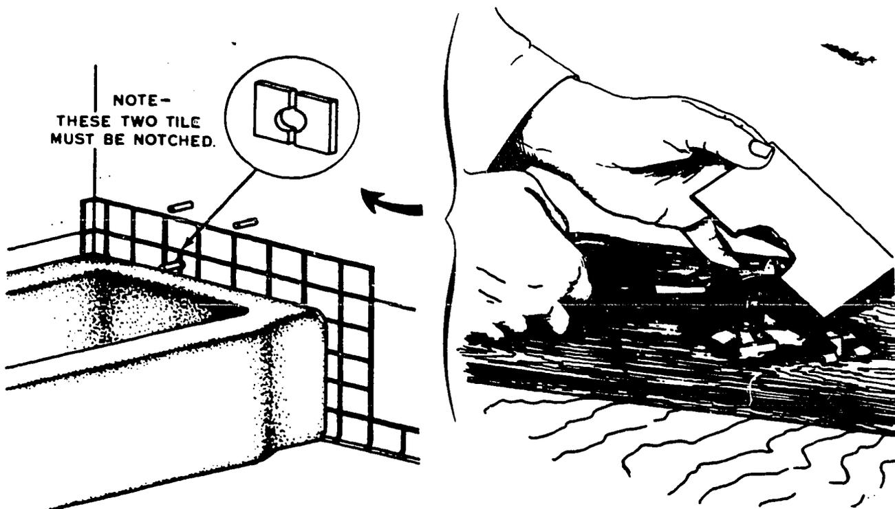
Figure 41. Adjusting a Tile to Fit Around a Pipe with Tile Nippers
