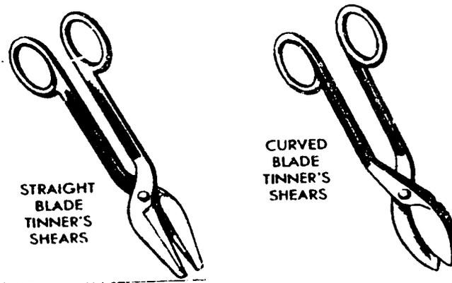
FIGURE 82. Metal Cutting Shears
