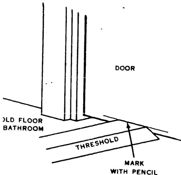
Figure 54. Marking the Door
