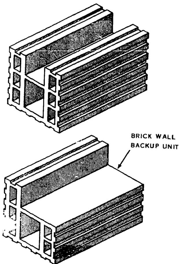
Figure 2. Structural Clay Tile
