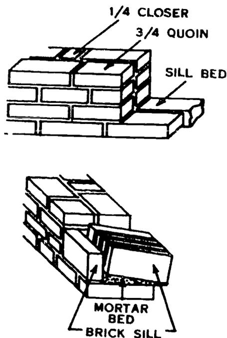
Figure 12. Constructing a Brick Window Sill
