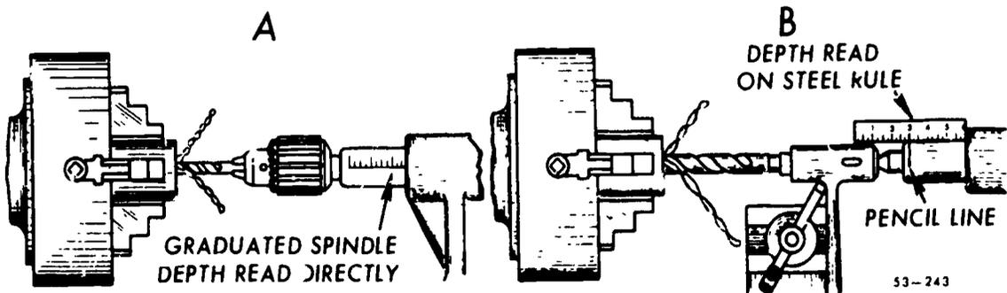
Figure 108. Measuring drill depth.
