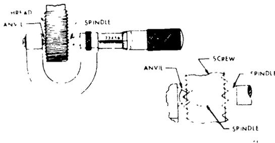
Figure 129. Measuring threads with a thread micrometer.
