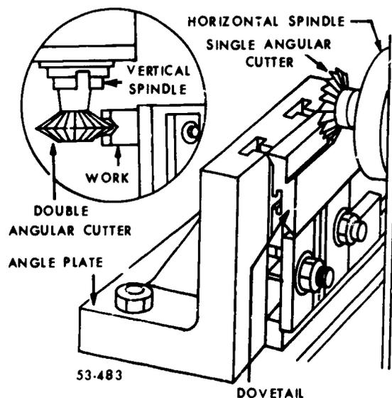
Figure 52. Angular milling.
