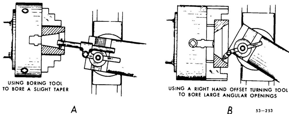
Figure 118. Boring short tapers.
