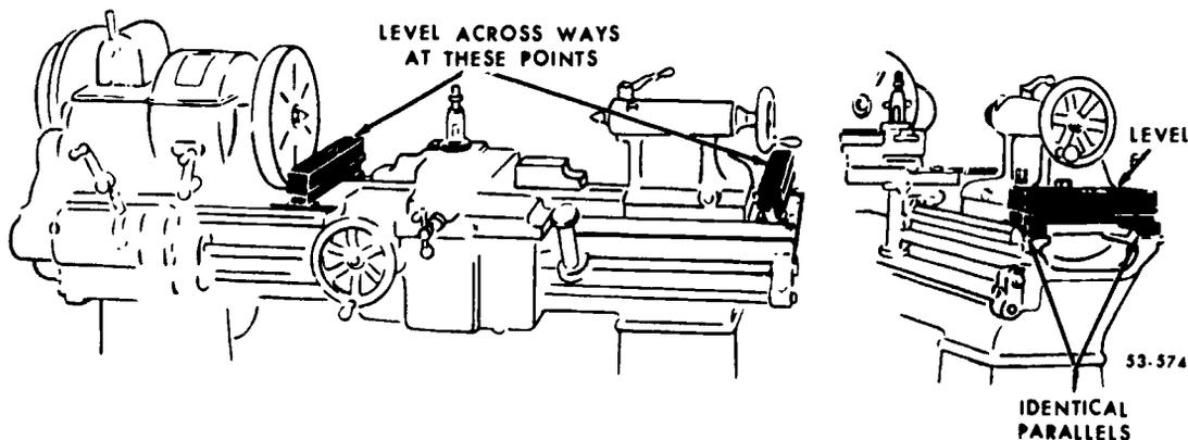
Figure 146. Placement of levels on lathe.
