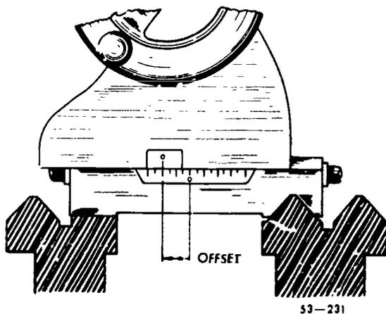
Figure 96. Tailstock cricket marks.
