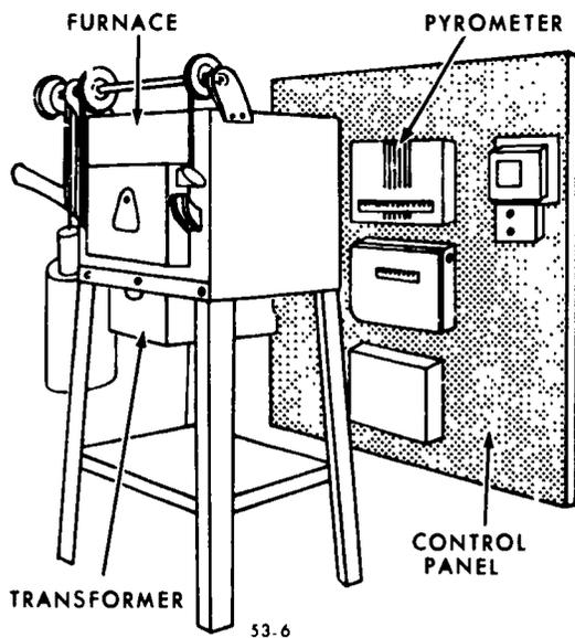
Figure 6. Electric furnace.
