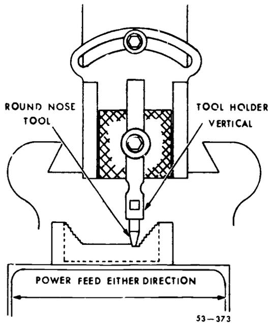
Figure 53 Roughing excess between two shoulders.
