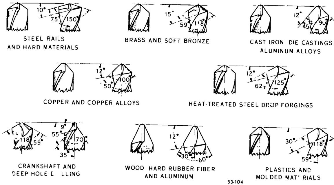
Figure 104. Drill point shapes.
