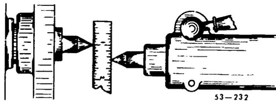
Figure 97. Measuring offset with a steel rule.
