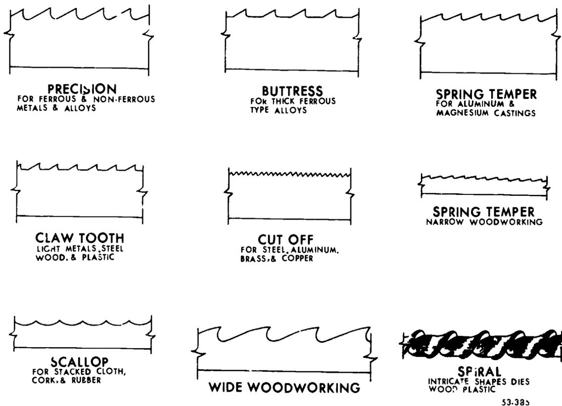
Figure 66. Shapes of saw band teeth.
