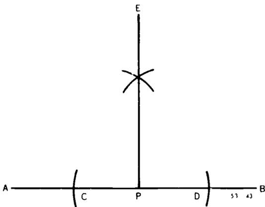
Figure 43. Erecting a perpendicular from a point on a line.
