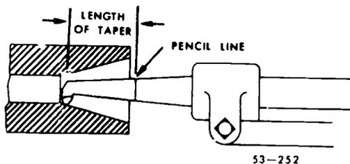
Figure 117. Marking boring bar.
