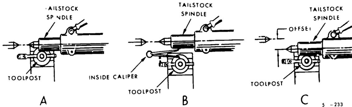
Figure 98. Measuring offset with inside calipers.
