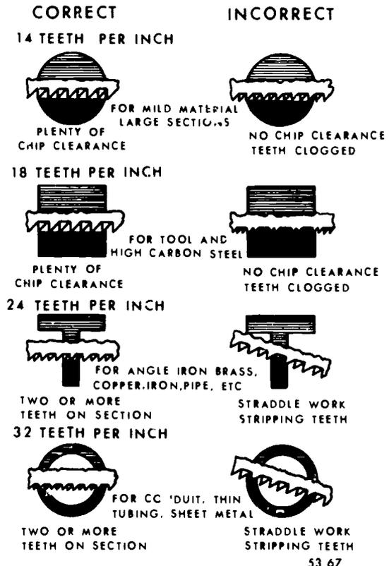
Figure 67. Section of pitch.
