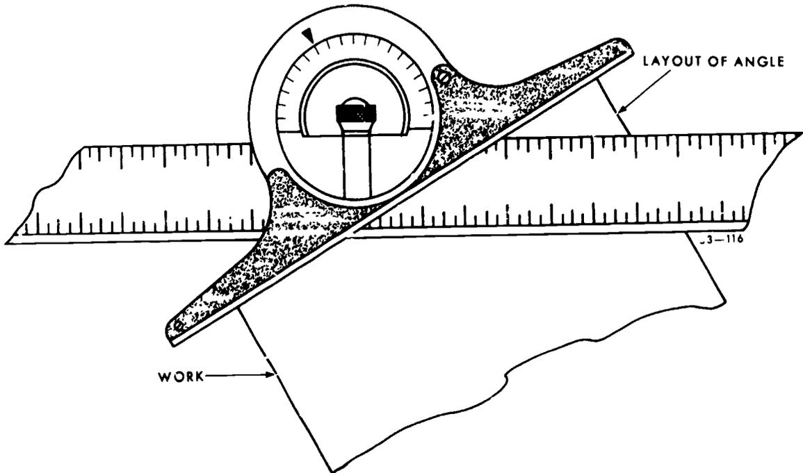
Figure 116. Use of protractor head.
