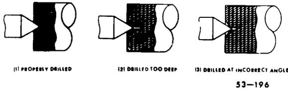
Figure 61. Correct and incorrect center holes
