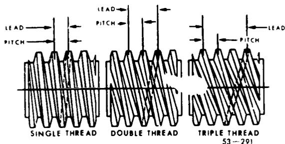
Figure 156. Comparison of single- and multiple-lead threads
