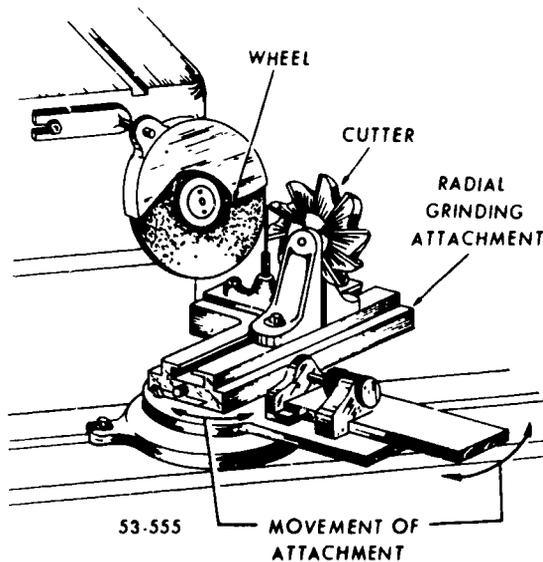
Figure 117. Radial grinding setup.
