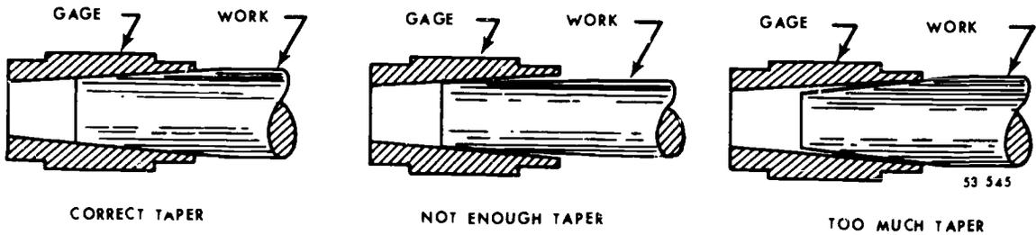
Figure 107. Checking taper using a taper gage.
