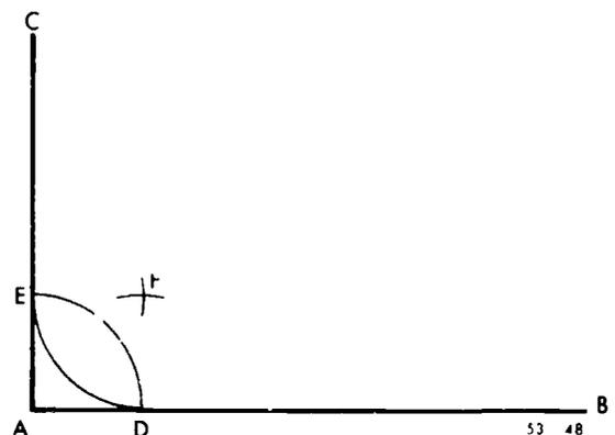
Figure 48. Constructing an arc within a right angle.
