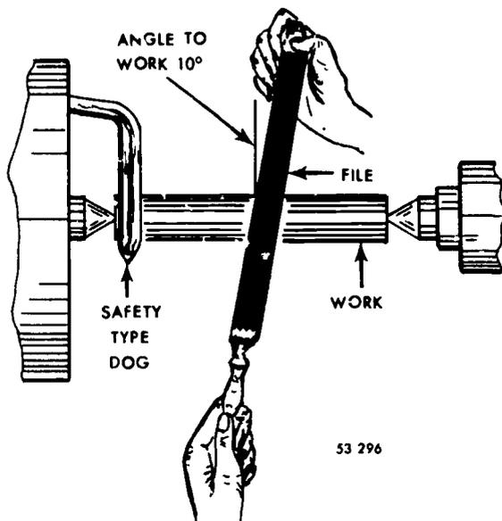
Figure 161. Filing work on a lathe.
