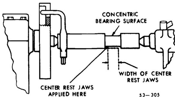
Figure 170. Concentric bearing surface.
