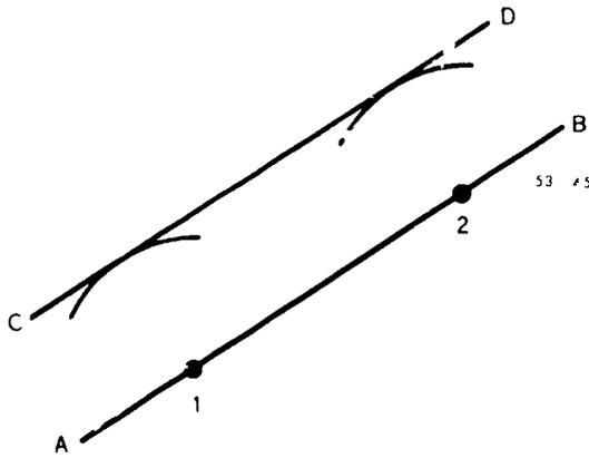
Figure 45 Constructing a line parallel to a line
