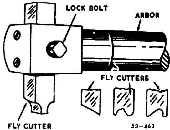
Figure 32. Fly cutter arbor and fly cutters.
