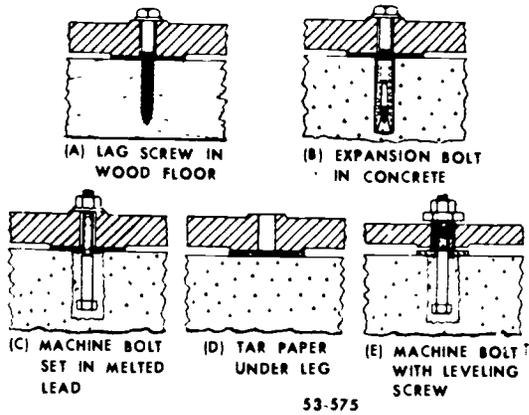
Figure 147. Fastening devices for securing machines.
