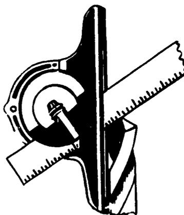
CHECKING DRILL POINT WITH PROTRACTOR
