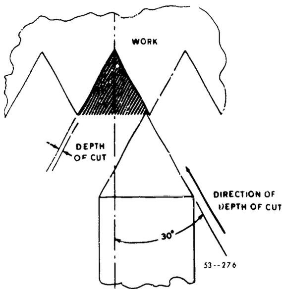
Figure 141. Action of threading tool.
