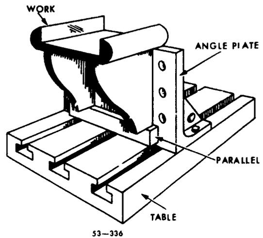
Figure 17 Nonadjustable angle plate.
