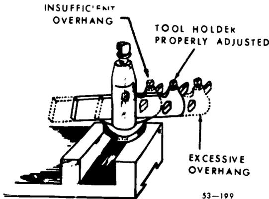
Figure 64. Toolholder overhang.
