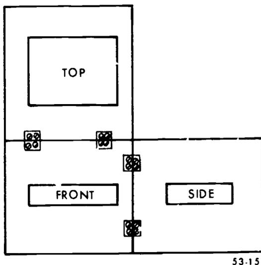
Figure 15. Orthographic projection onto paper.
