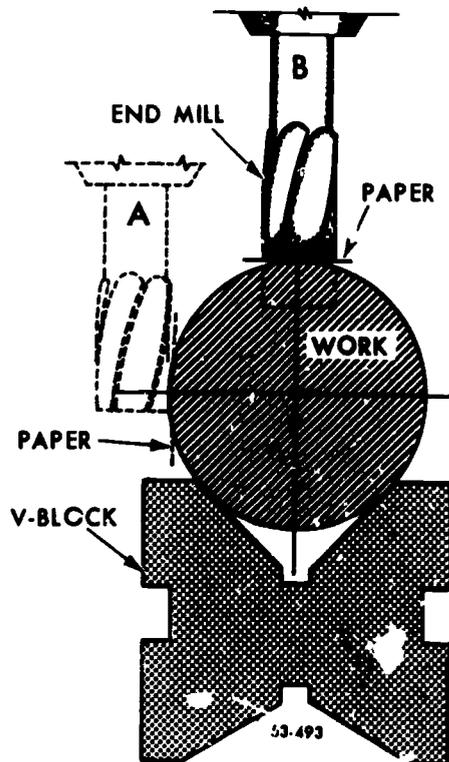
Figure 62. Alining an end mill with the work.
