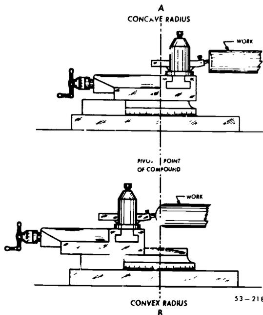
Figure 83. Machining a radius with the compound rest.
