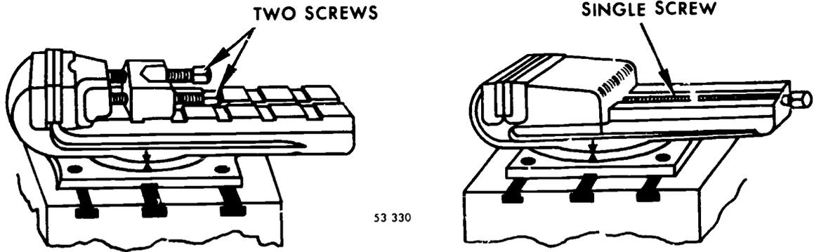
Figure 11. Double and single screw vises.
