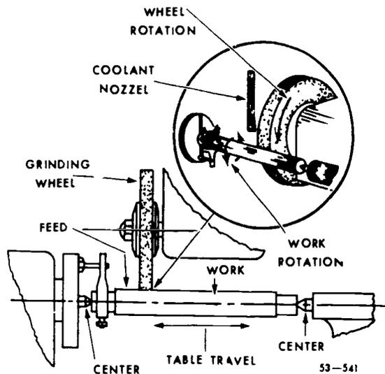
Figure 103. Cylindrical grinding.
