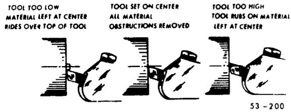
Figure 65. Effect of facing tool height.
