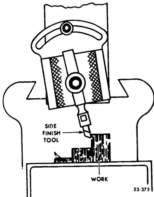
Figure 55. Position of side finishing tool.
