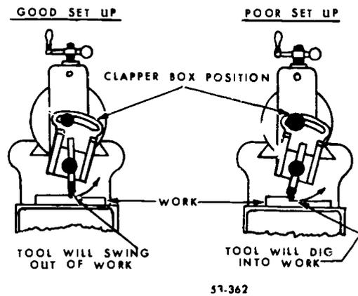
Figure 42. Positioning the tool and clapper box.
