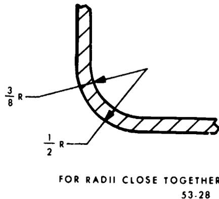
Figure 28. Dimensioning arcs and radii.
