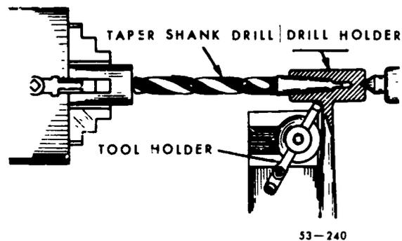
Figure 105. Drill holder floated on the dead center.
