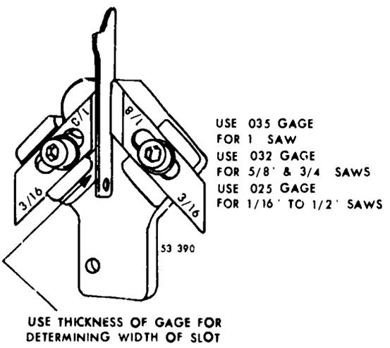
Figure 71. Installing right insert.
