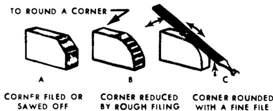
Figure 63. Rounding corners and drawfiling.
