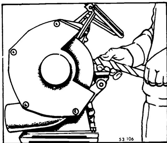
Figure 106. Grinding a drill.
