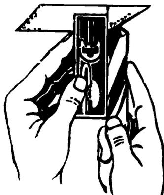
CHECKING DRILL POINT WITH DRILL GAGE
