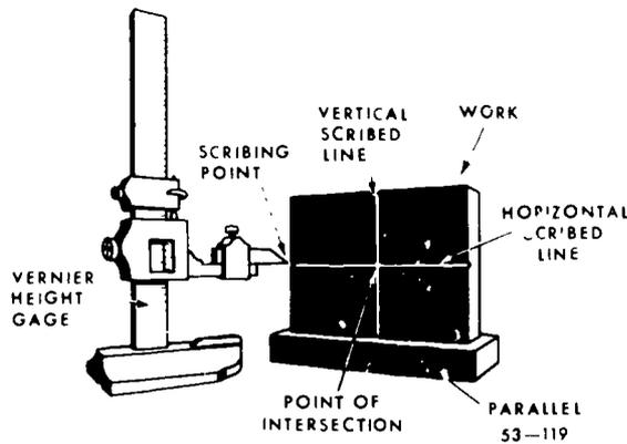
Figure 119. Vernier height gage.
