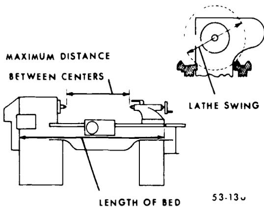
Figure 1. Size designation of a lathe.
