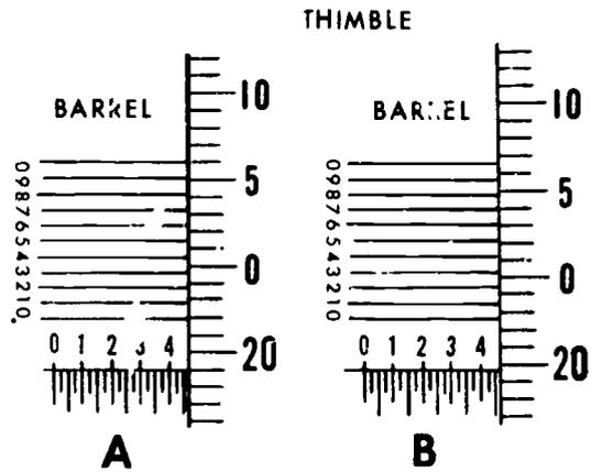
$$\begin{aligned} & .4690'' \\ & .0007 \\ \text{READING} = & .4697 \end{aligned}$$
