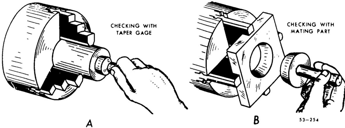
Figure 119. Checking internal tapers.
