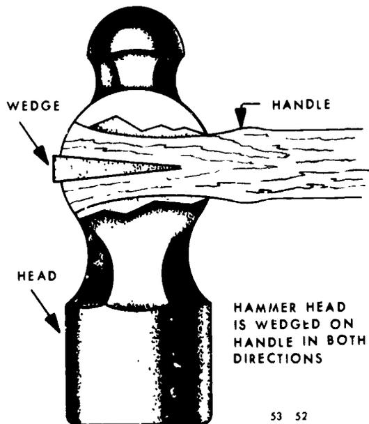
Figure 52. Securing head on handle.
