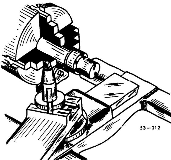
Figure 77. Parting setup.
