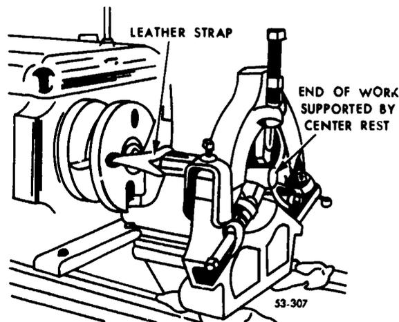
Figure 172. Tying the lathe dog.
