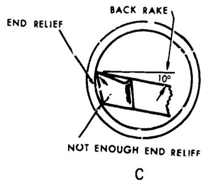
Figure 113. Boring tool angles.
