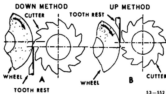
Figure 114. Cutter sharpening positions.
