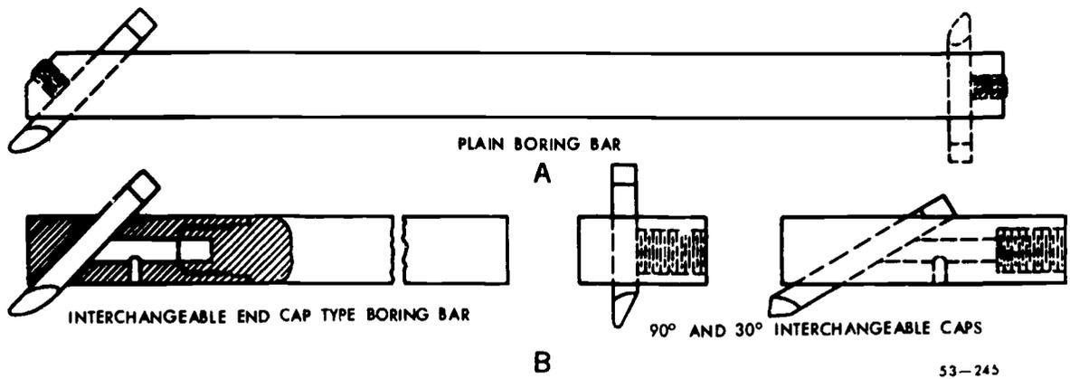
Figure 110. Types of boring bars.
