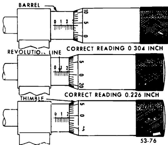
Figure 76. Micrometer readings.
