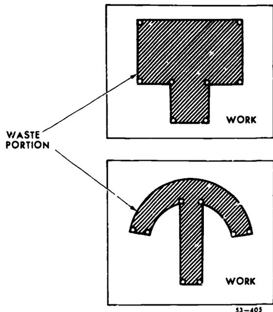
Figure 86. Internal contour.
