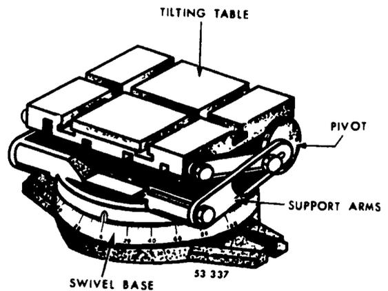
Figure 18. Adjustable angle plate
