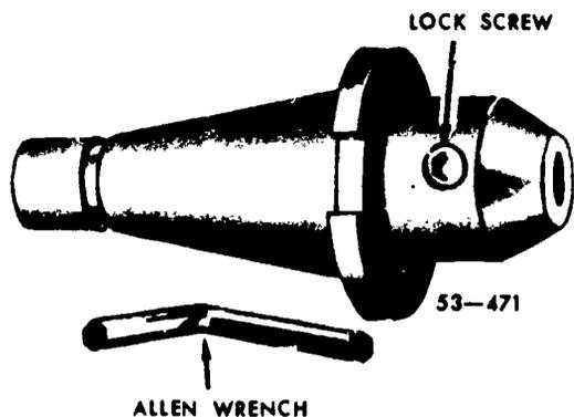
Figure 40. Cutter adapter.
