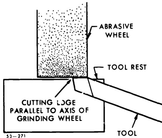
Figure 136. Grinding side rake.
