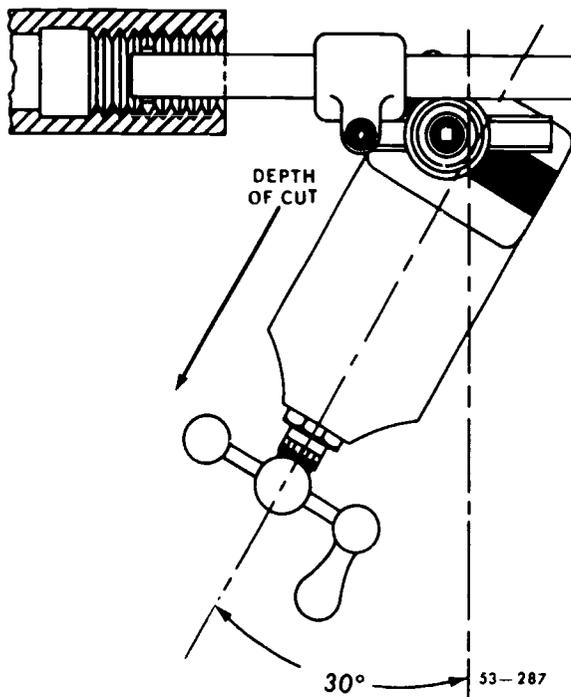
Figure 152. Position of compound rest for internal threads.
