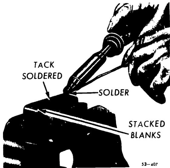
Figure 96. Compressing and soldering small objects
