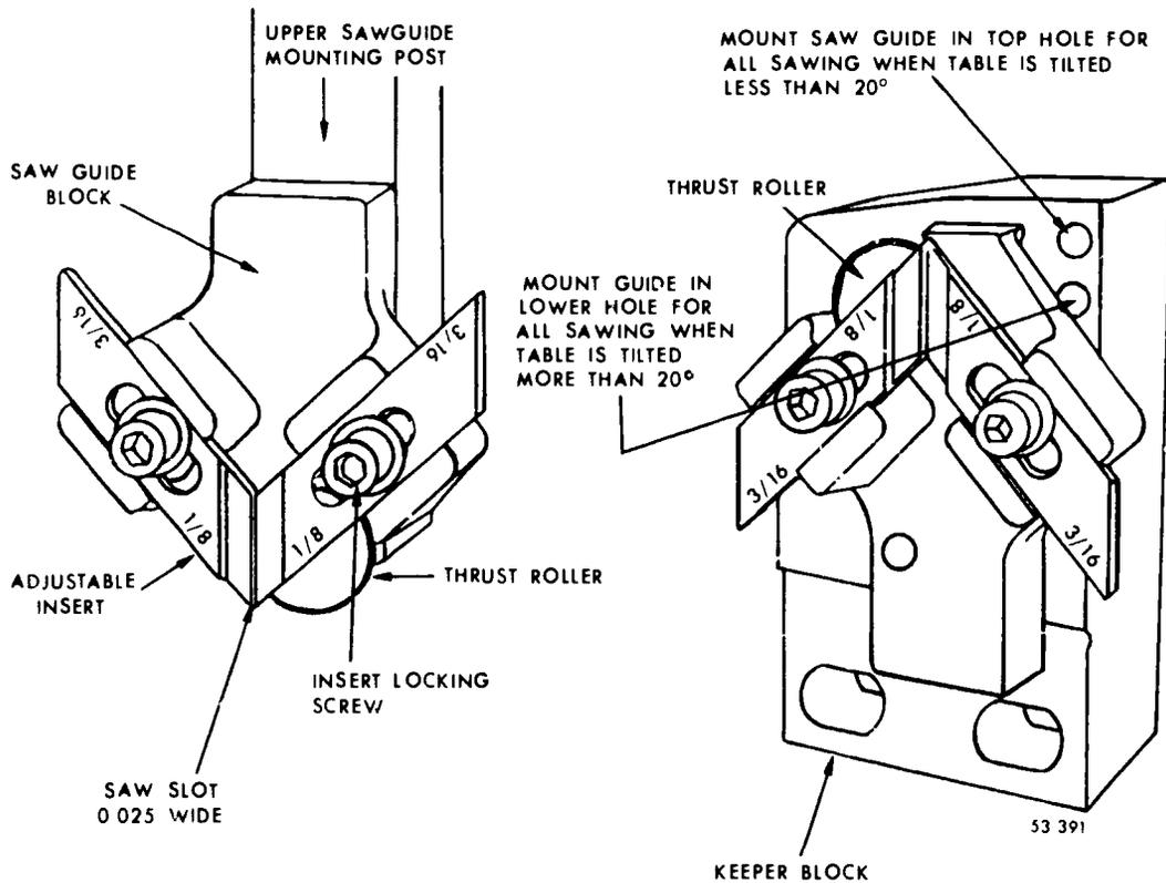
Figure 72. Mounting saw guides
