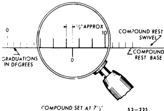
Figure 90. Determining fractional setting of compound rest.
