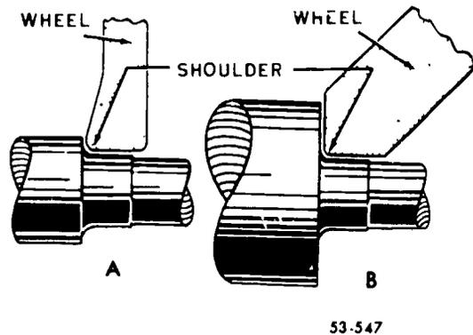
Figure 109. Shoulder grinding setups.
