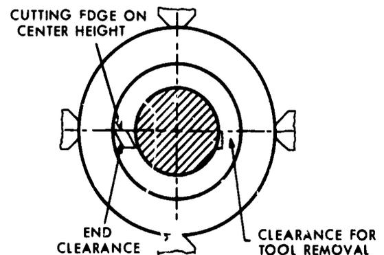
Figure 149. Position of internal threading tool.
