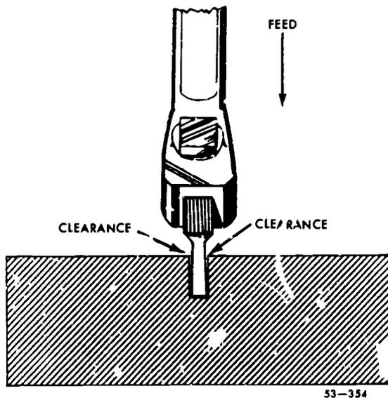
Figure 34. Cutting off tool.
