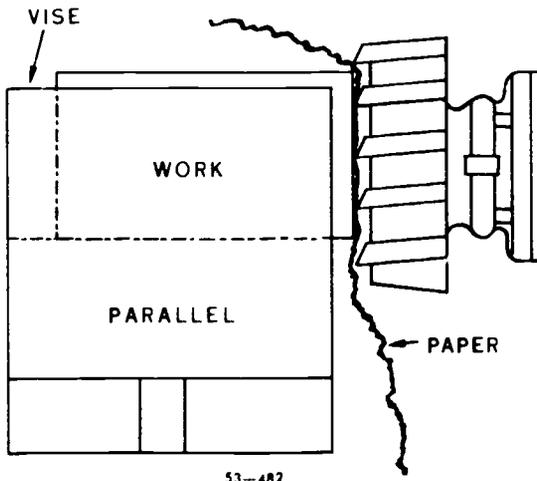
Figure 51. Picking up the work surface.
