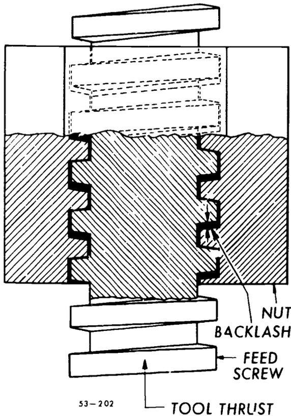
Figure 67. Backlash between feedscrew and nut.
