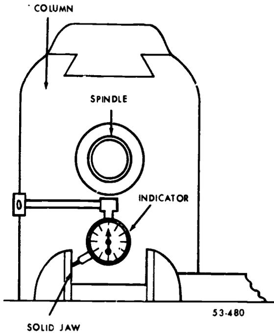
Figure 49. Alining vise jaws using an indicator.
