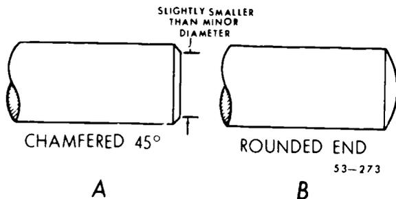
Figure 138. End of work prepared for threading.
