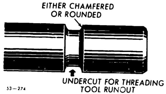
Figure 139. Undercut for threading tool runout.
