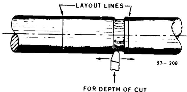
Figure 73. Undercutting a shaft.
