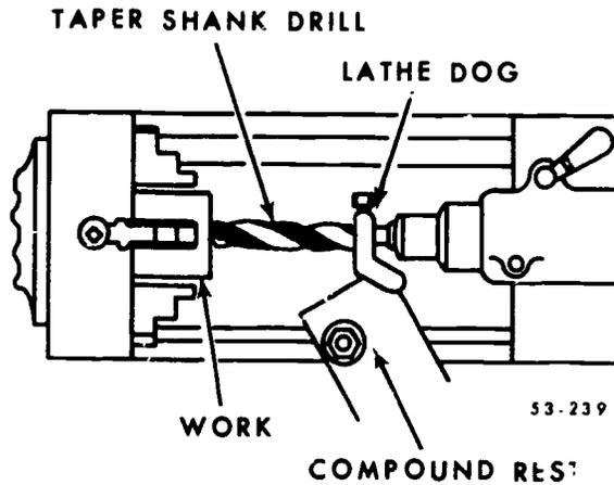
Figure 104. Supporting a drill in the tailstock spindle.
