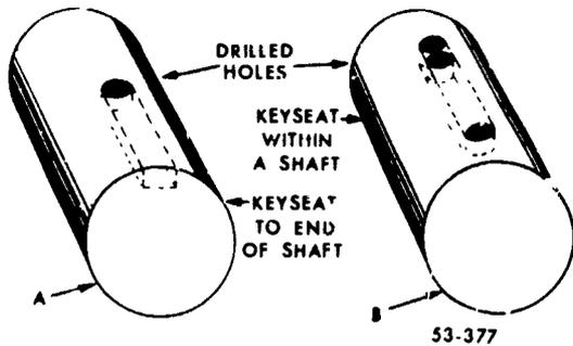
Figure 58. Drilled holes for keyseats.
