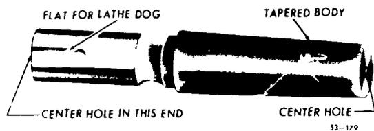
Figure 44. Tapered plug mandrel.
