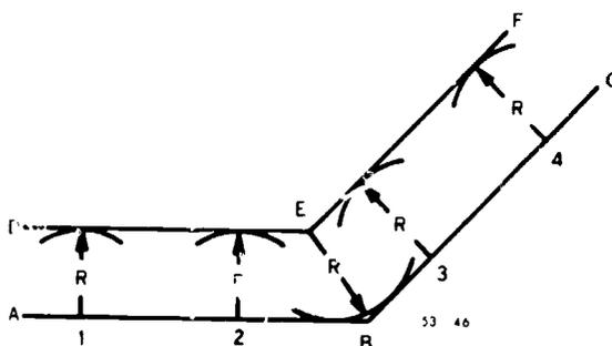
Figure 46. Constructing an arc tangent to intersecting lines.
