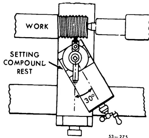
Figure 140. Position of compound rest.
