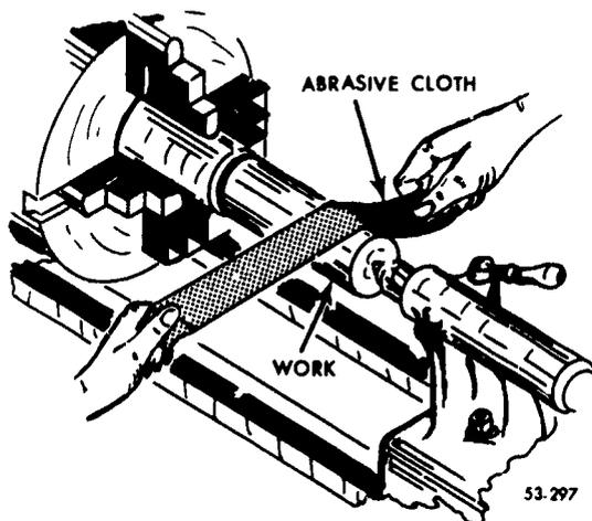
Figure 162. Polishing work on a lathe.
