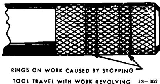
Figure 167. Rings on a knurled surface.
