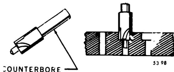
Figure 98. Counterbore and counterbored hole.
