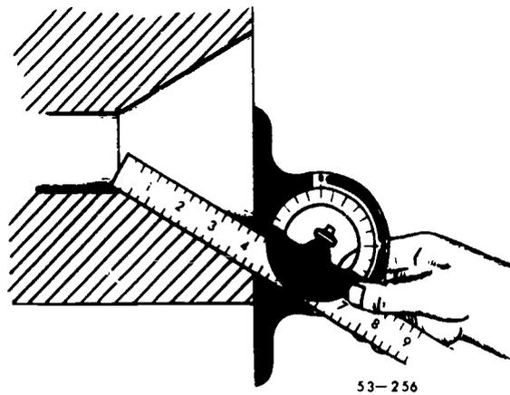
Figure 121. Measuring taper angle with a protractor.
