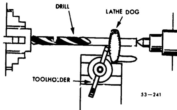
Figure 106. Drill floated on the dead center.
