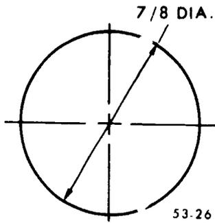
Figure 26. Dimensioning large diameters.
