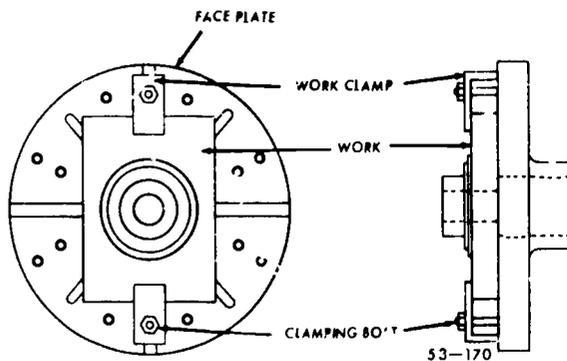
Figure 35. Work clamped on faceplate
