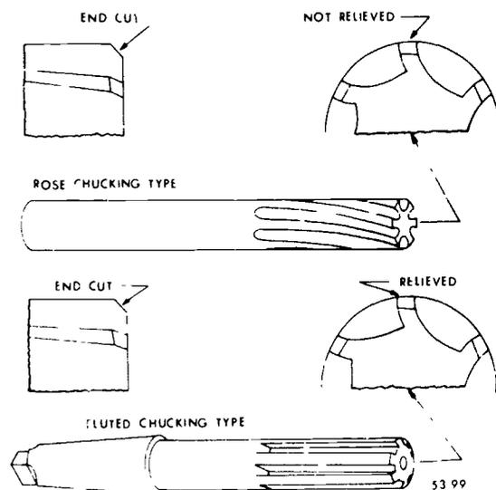
Figure 99. Machine reamers.
