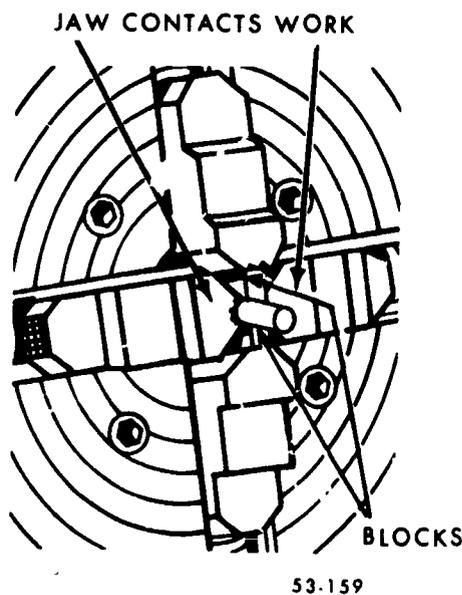
Figure 24. Small work held in a four-jaw chuck.
