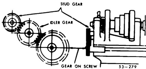
Figure 144. End gearing.
