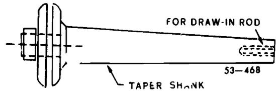
Figure 37. Screw slotting cutter arbor.
