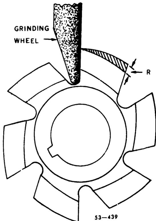
Figure 8. Sharpening formed cutters.
