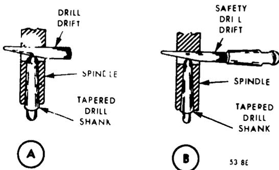
Figure 88. Using drill drifts.
