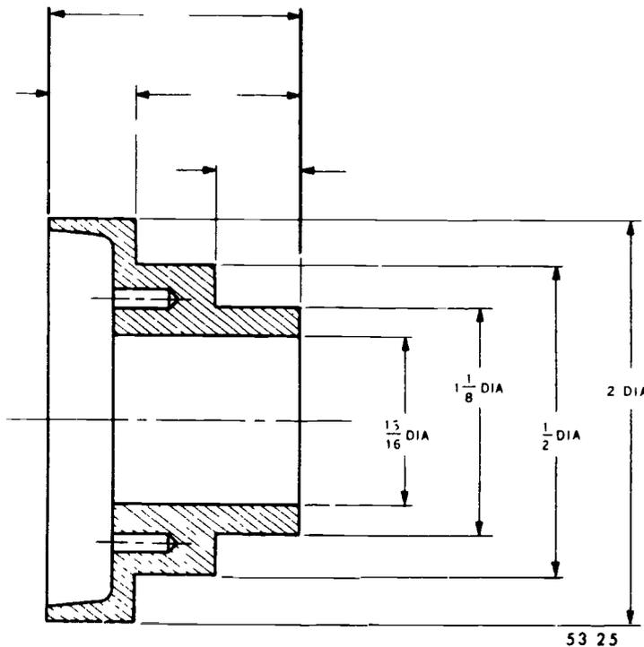
Figure 25. Dimensioning methods shown in profile.
