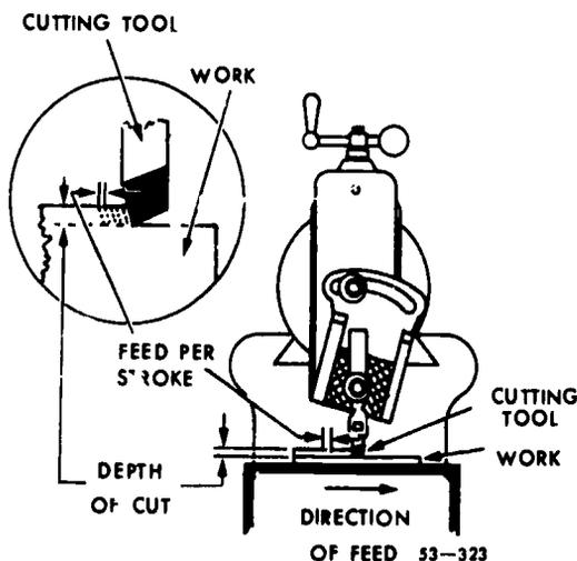
Figure 4. Shaper feed and depth of cut.
