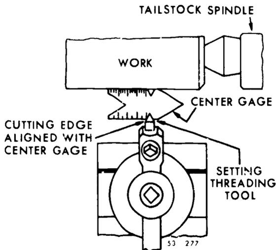
Figure 142. Positioning threading tool
