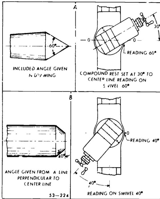
Figure 89. Setting the compound rest.
