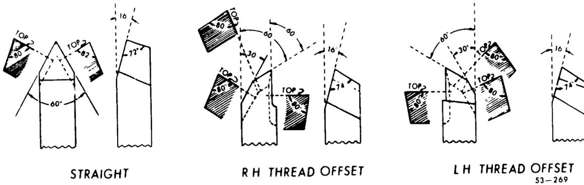
Figure 134. Straight and offset threading tools.
