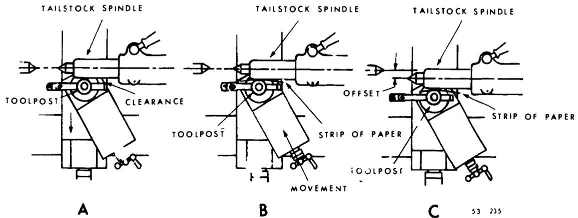
Figure 100. Measuring offset with the cross-slide graduated collar.
