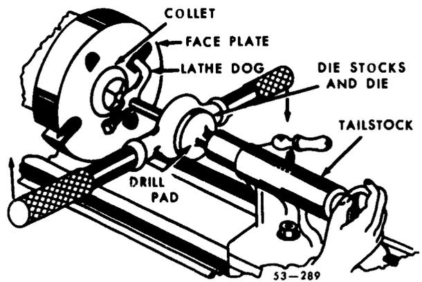
Figure 154. Die threading setup.
