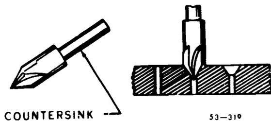
Figure 97. Countersink and countersunk hole.
