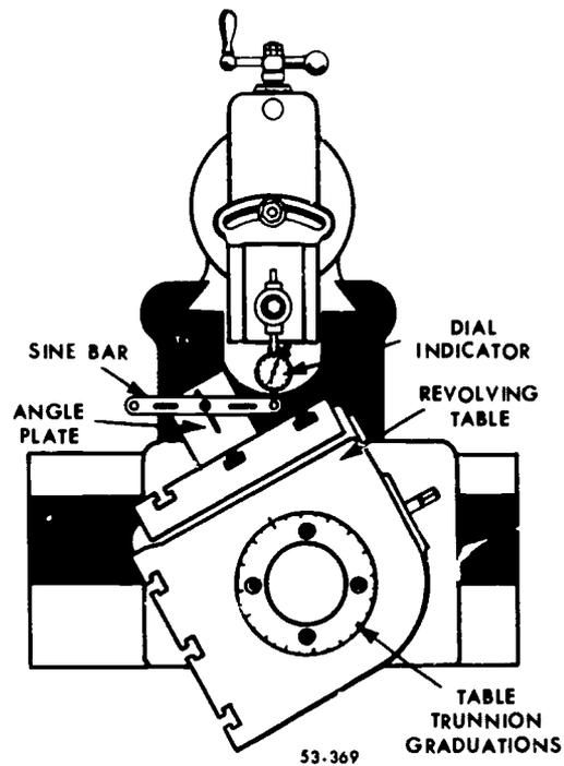
Figure 49. Alining table with a sine bar.
