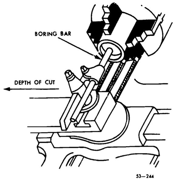
Figure 109. Boring in the lathe.
