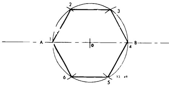
Figure 49. Constructing a regular hexagon.
