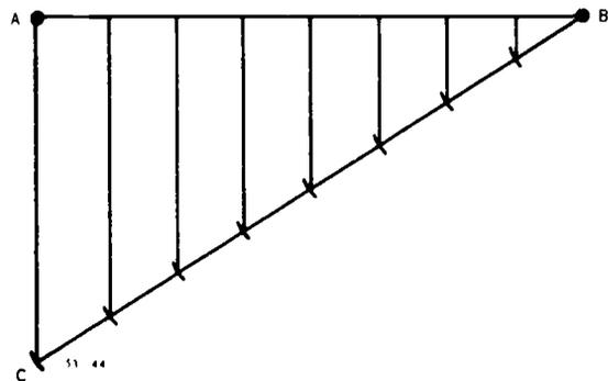
Figure 44. Dividing a line into equal parts.
