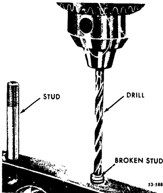
Figure 135. Drilling a broken stud.
