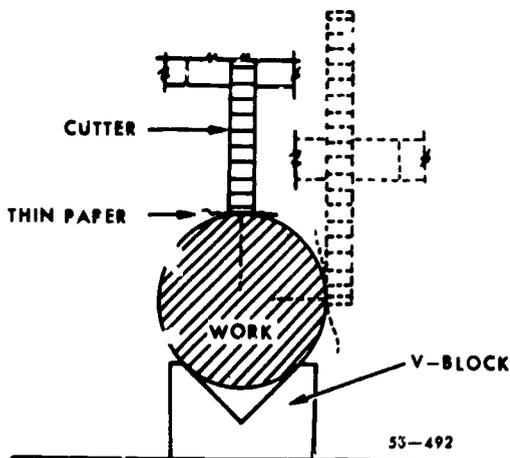
Figure 61 Alining cutter using a paper strip.
