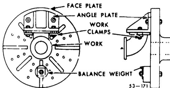
Figure 36. Work mounted on an angle plate.
