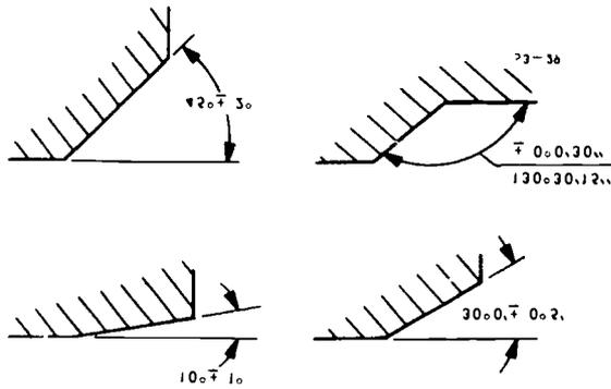
Figure 29. Dimensioning angles and chamfers.
