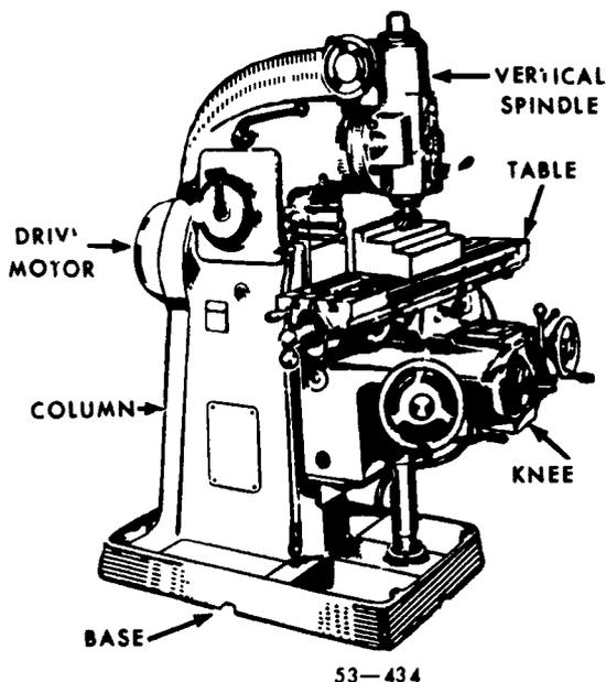
Figure 4. Vertical spindle milling machine.
