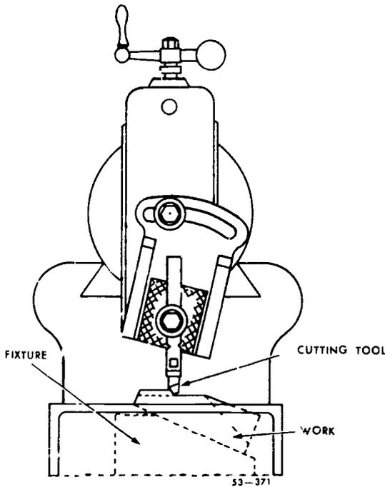
Figure 51. Angular planing with a fixture.
