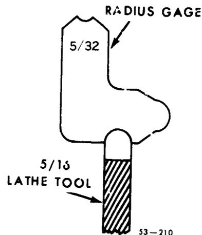
Figure 75 Forming tool ground to fit radius gage.
