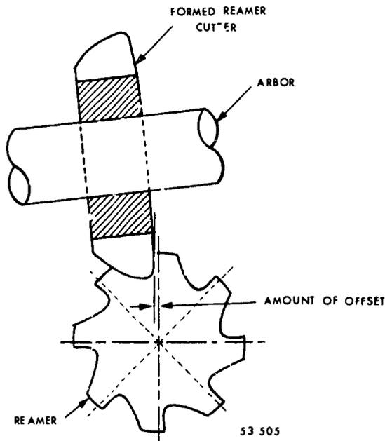
Figure 69 Negative rake tooth.
