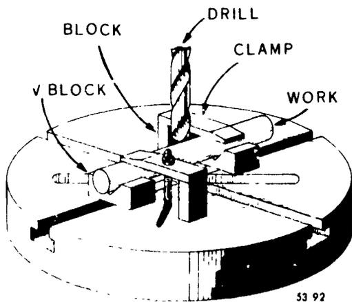
Figure 92. Work clamped to table.
