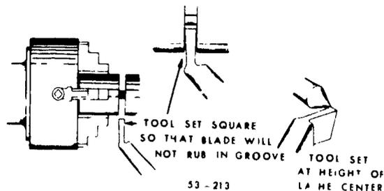
Figure 78. Position of a parting tool.
