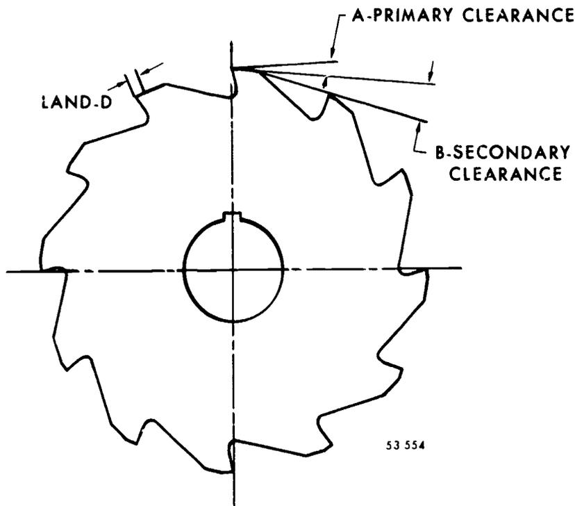
Figure 116. Recommended clearance angles.
