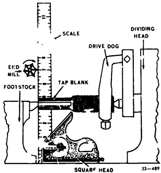
Figure 58. Alining the work and cutter.
