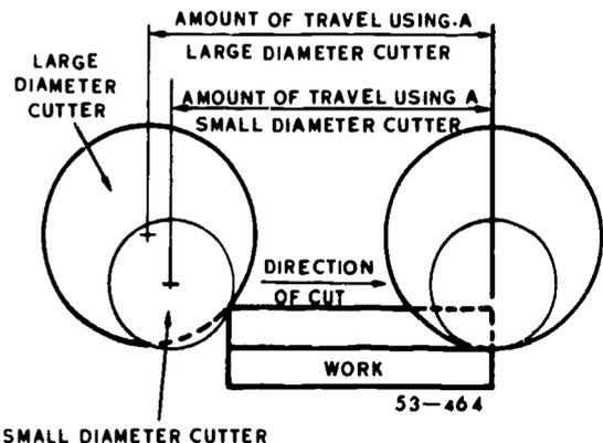
Figure 33. Cutter diameter selection.
