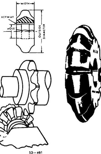
Figure 30. Sprocket wheel cutter.
