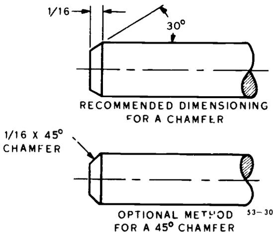
Figure 30. Methods of dimensioning chamfers.
