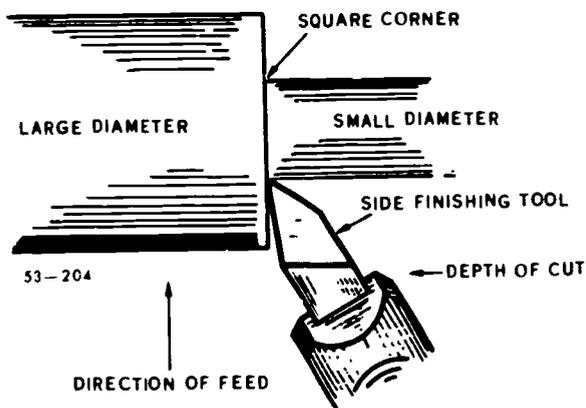
Figure 69 Squaring a shoulder with a side finishing tool.
