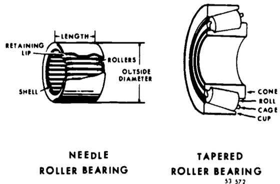
Figure 132. Needle and tapered roller bearings.
