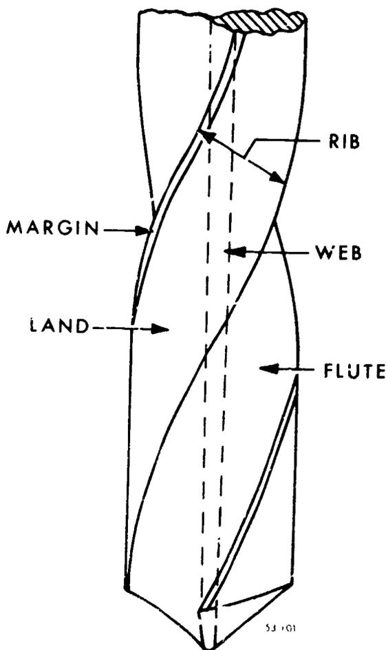
Figure 100 Body parts of a twist drill.
