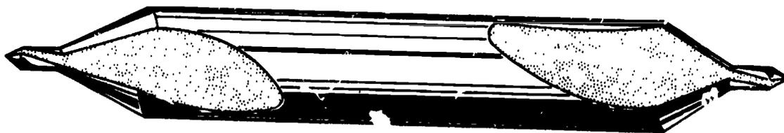
Figure 96. Combination drill and countersink (center drill).
