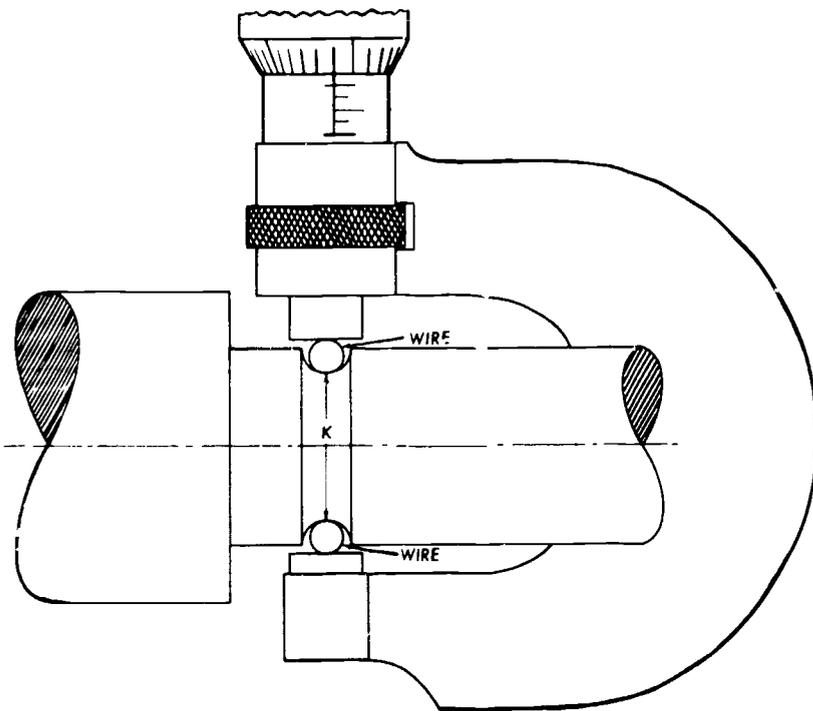
MICROMETER READING =  $K + 2(\text{WIRE DIA})$
