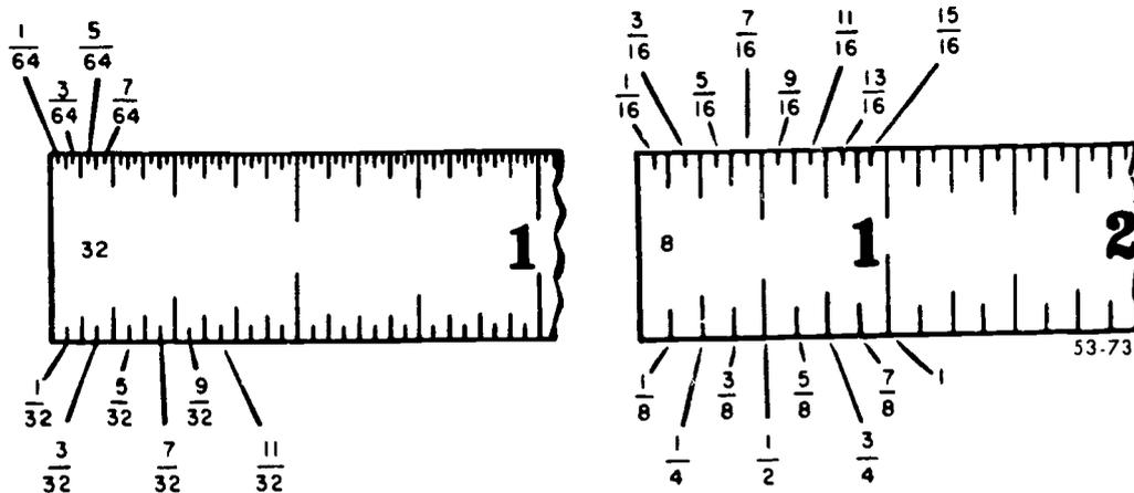
Figure 73. Typical scale graduations.
