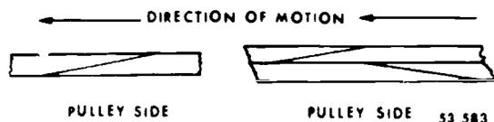
Figure 152. Flat belt lap joint.
