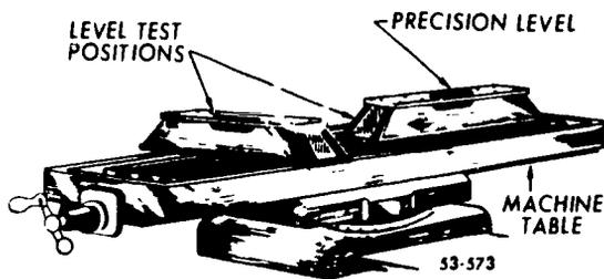
Figure 145. Placement of levels on milling machine.
