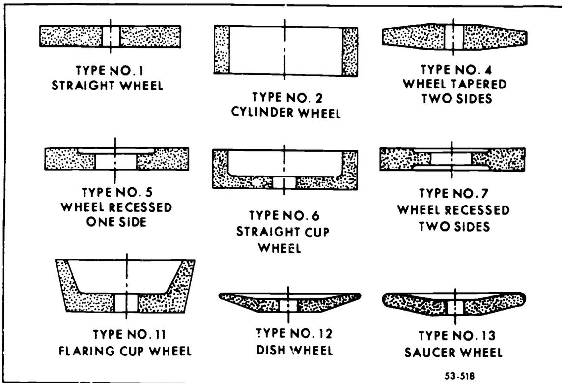
Figure 83. Standard grinding wheel shapes.
