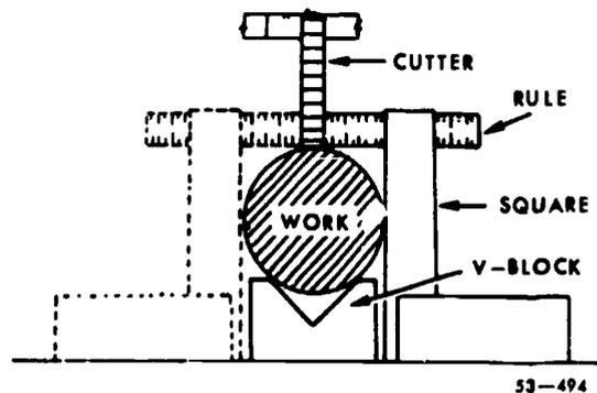
Figure 63. Visual alignment of a cutter.
