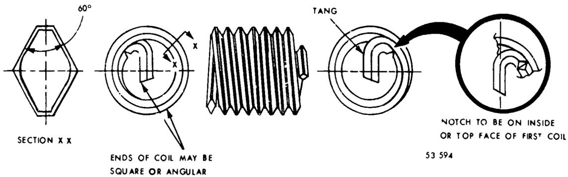
Figure 141. Diagram of a heli-coil insert.
