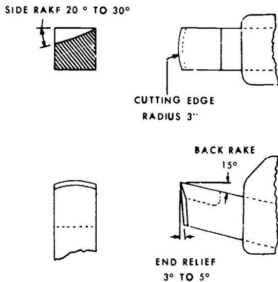
Figure 26. Shear tool for steel.
