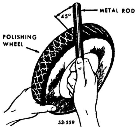
Figure 120. Breaking a polishing wheel.
