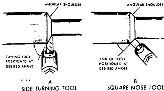
Figure 71. Machining an angular corner.
