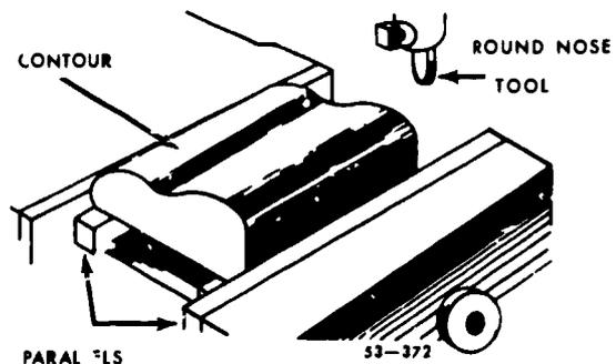
Figure 52. Machining a contour.
