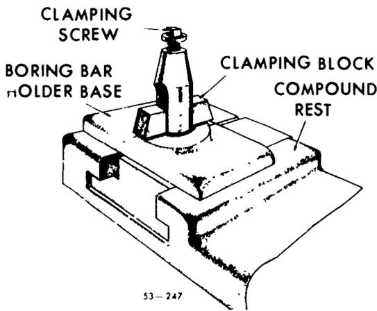
Figure 112. Use of the clamping block.
