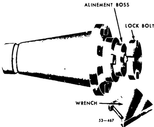
Figure 36. Shell end mill arbor.
