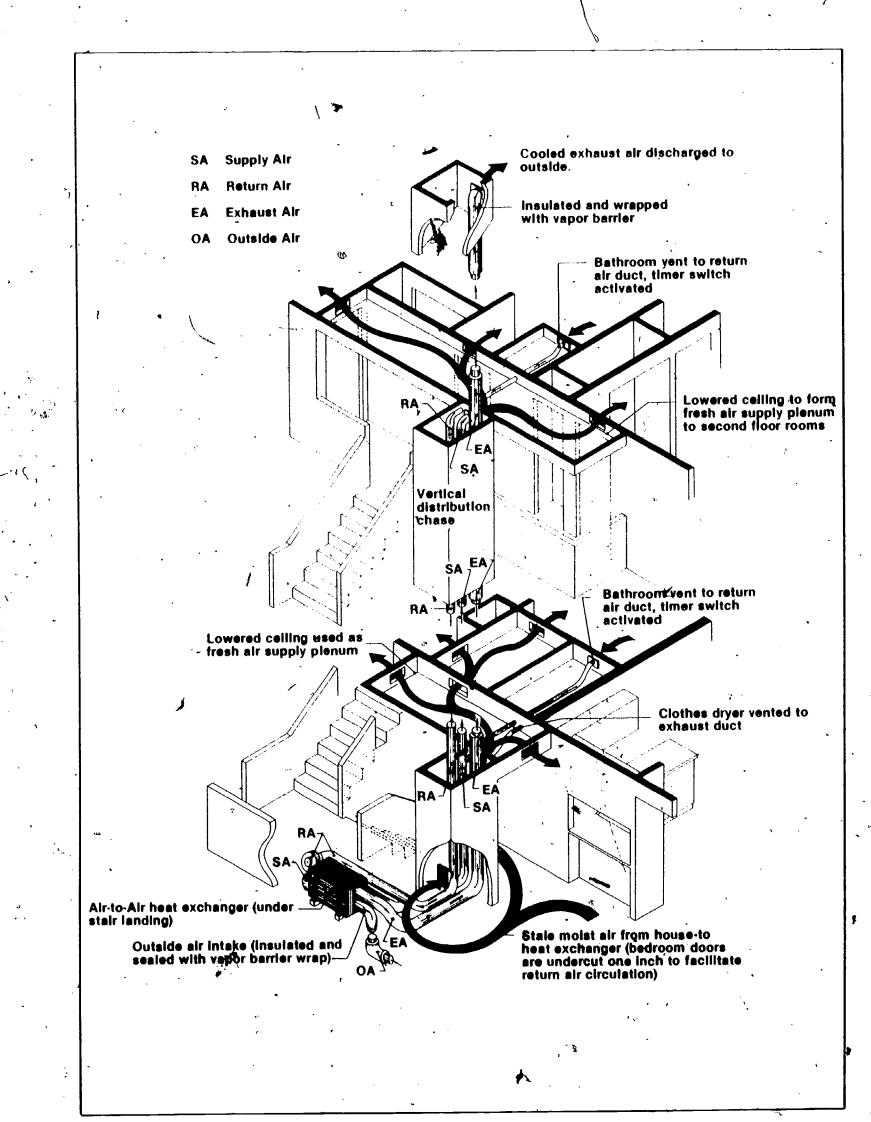
FIGURE 7: This isometric cutaway shows how the integration of a central, ducted air-to-air heat exchanger is best accomplished during the design phase. The system shown is for a two-story house.
