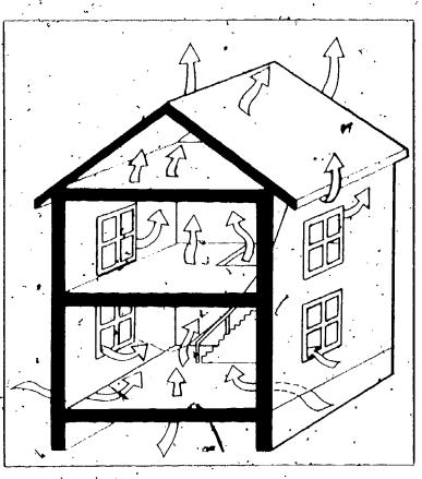
FIGURE 3: The "stack effect" is one significant way in which conventionally, built houses lose heated air through infiltration and exfiltration.
