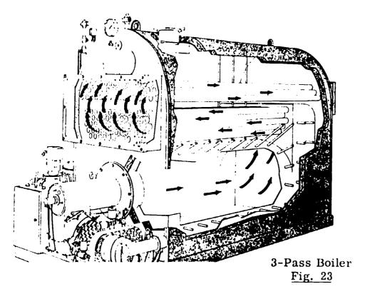
The large stayed firebox of this 3-pass unit has an arched crown sheet; the rear reversing chamber has stayed waterlegs at sides with a submerged top. Flow is forward in short second-pass tubes, to the rear in the longer third-pass tubes. This furnace shape requires stays, as do the waterlegs at the sides of the rear chamber into which the firebox discharges. Here the aim of the designer is for a large combustion space and a higher ratio of furnace-to-tubular surface.
