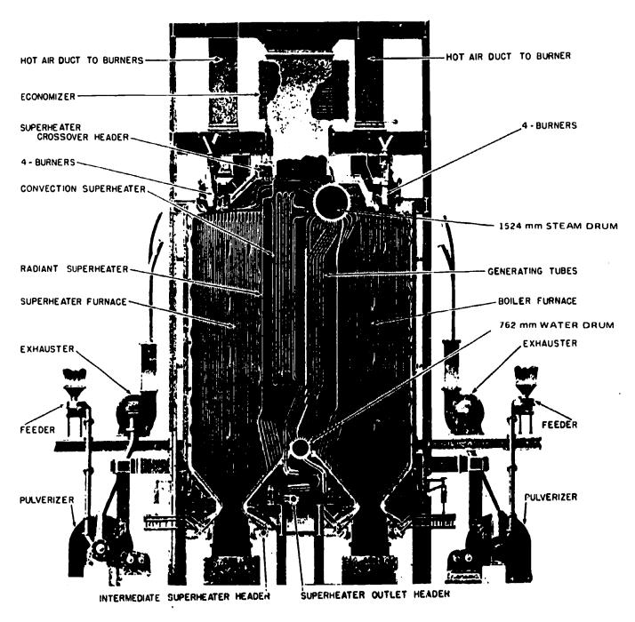
Twin Furnace - Differentially Fired (Foster Wheeler Ltd.)
