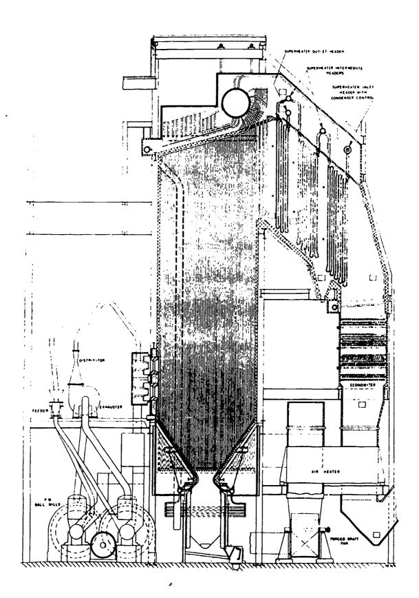
Steam Generator with Vertically Arranged Air Heater  $\underline{\text{Fig. 42}}$
