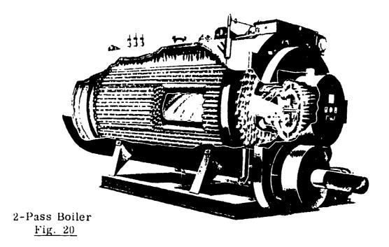
The first pass in this unit is a centrally-located corrugated furnace with a spinning flame pattern. The second pass consists of a multiplicity of tubes in a staggered layout. "Impellers" at tube entrances impart spiral gas action.
