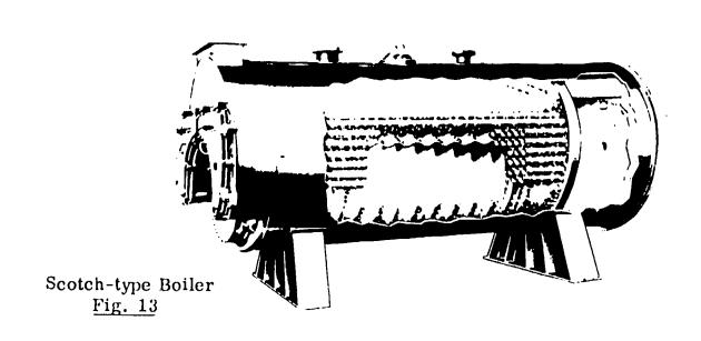
This type of boiler employs welded construction. Combustion occurs in the corrugated internal furnace; dryback refractory-lined rear chamber reverses flow, directs gas forward through tubes to smoke-box at the front.
