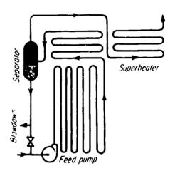
In once-through designs there is no recirculation; feedwater leaves the tubes as steam. When pressures are below critical, a separator may be used to remove any moisture present in steam.
