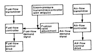
Metering Control Parallel Arrangement
