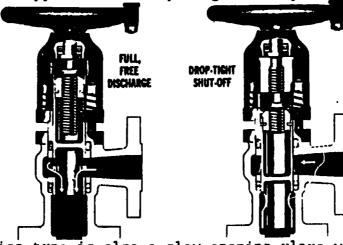
The seat and disc type is also a slow opening vlave with a bottom disc that closes the valve. It is a handwheel operated valve.
