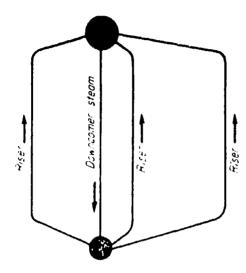
In actual natural-circulation units the principles of Figs. 4 and 5 apply, but there are usually many parallel riser circuits carrying steam-water mixture and several larger, cold downcomers.
