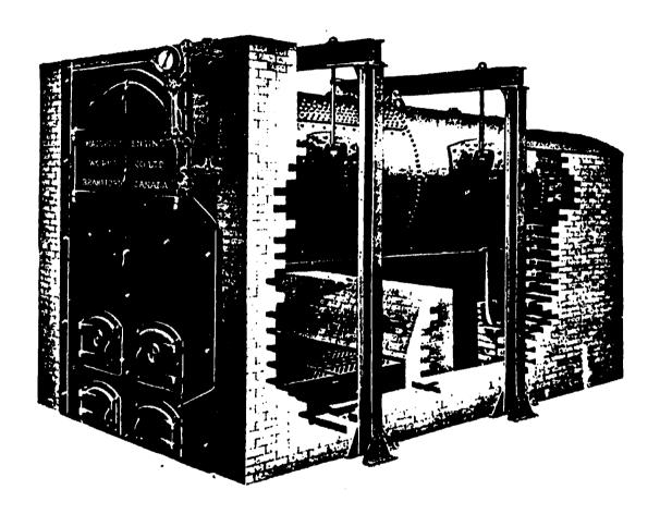
Suspension Method for H.R.T. Boiler Fig. 5
