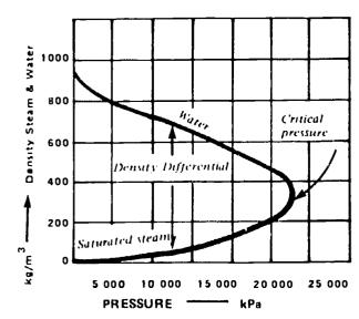
Pressure-Density Curve for Water and Steam Fig. 5
