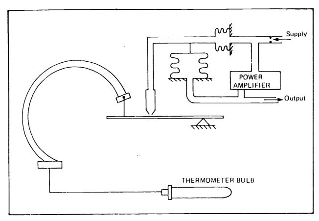
Pneumatic Temperature Transmitter
