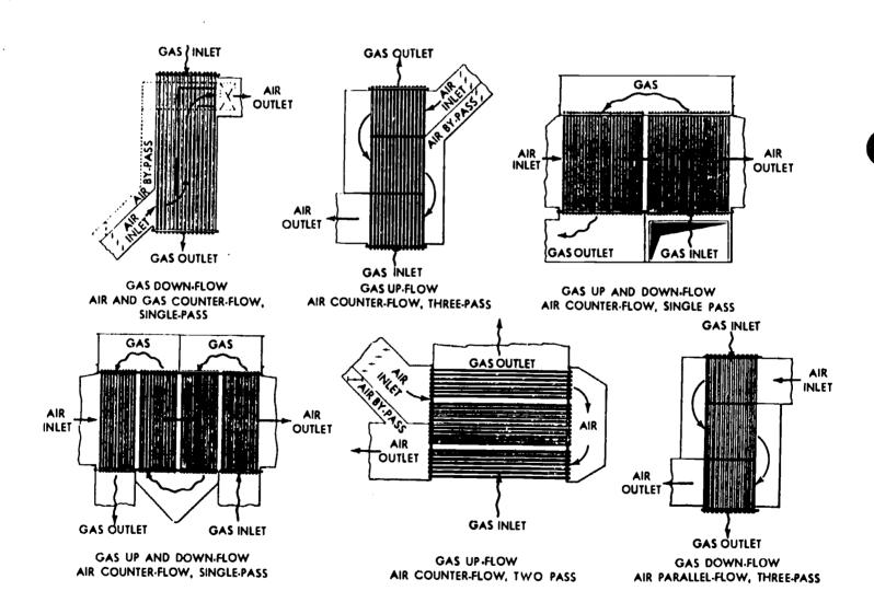
Tubular Air Heater Arrangements Fig. 38
