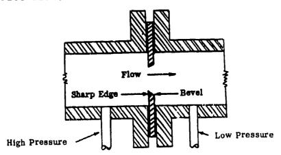
Orifice Plate with Pressure Taps
