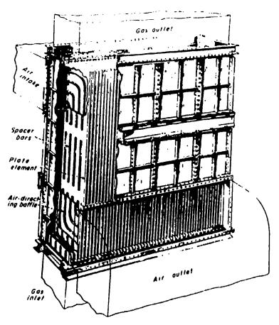
Plate Type Air Heater Fig. 37
