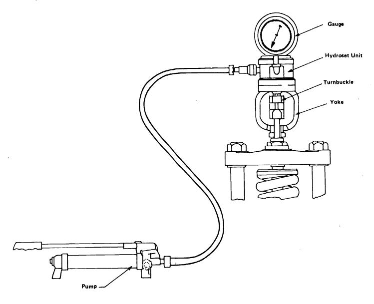
Safety Valve Hydraulic Testing (Dresser Industrial Valve and Instrument Division)
