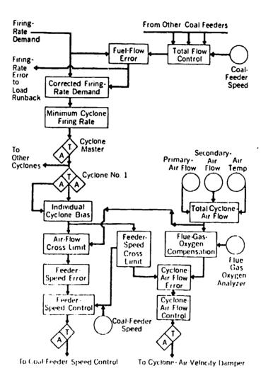
Combustion Control with Gas Analyzer (Babcock and Wilcox)
