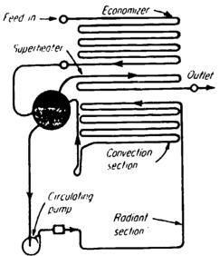
Forced circulation employs a pump to overcome resistances. It may be used at high pressures where natural circulation forces are small, or at lower pressures to give and dom in tube layout.
