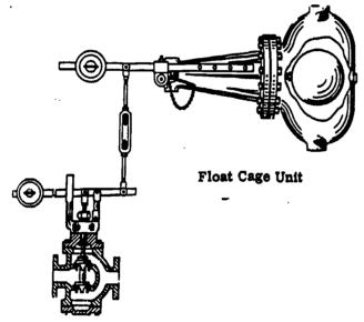
The <u>float manometer</u> is a differential pressure gauge. The manometer is attached to the top of the vessel. A mercury reservoir responds to the rise and fall of liquid in the vessel. The movement of the mercury moves a float which actuates the indicator.
