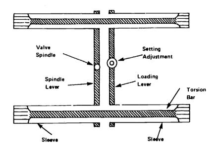
Torsion Bar, Lever and Sleeve Arrangement
