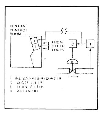
Fig. 18 shows a simple pressure control system where changes in the pressure within the pipe is sensed by a transmitter. The transmitter signal is sent to a controller and also to an indicator and recorder located in the control room. The controller, which is located adjacent to the control valve, causes the actuator to operate the valve in accordance to the pressure changes within the pipe.
