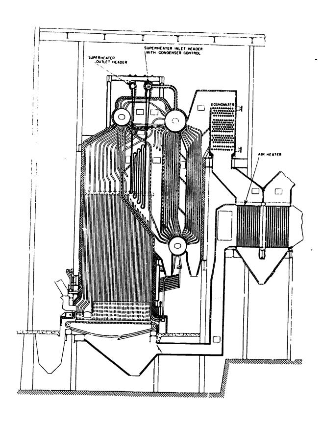
Steam Generator with Economizer and Tubular Air Heater  $\underline{\text{Fig. 39}}$
