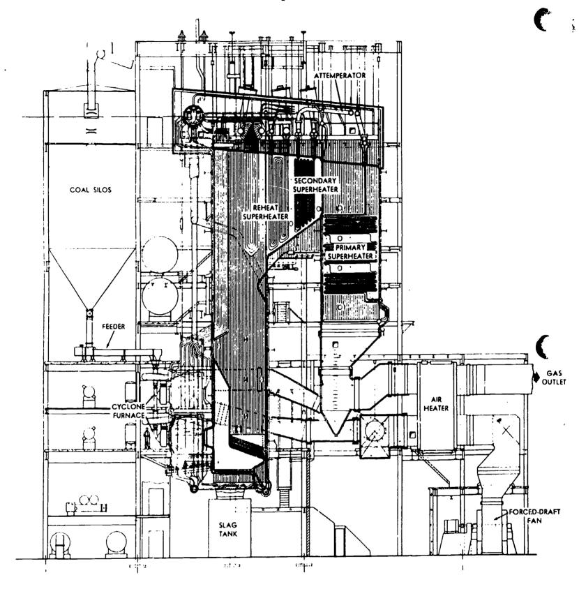
Watertube Steam Generator - pressurized Cyclone-furnace fired. Fig. 5
