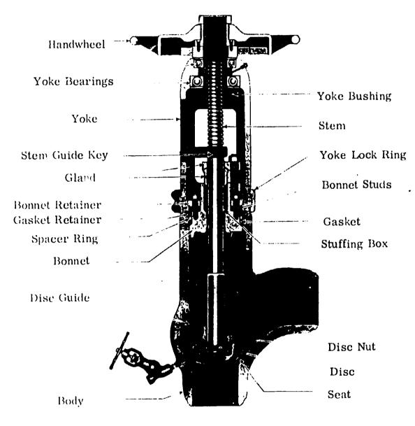
Angle Type Outside-Screw-and-Yoke Stop Valve (Edward Valves Inc.)
