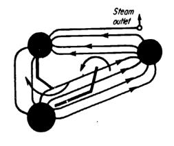
Circulation situation in a threedrum low-head boiler is more complicated. Downcomers are partially heated, there is less head difference to produce circulation, more frictional resistance.
