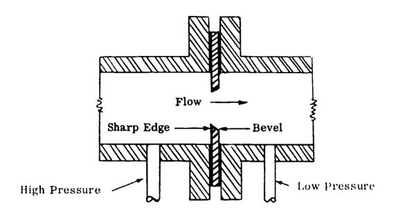
Orifice Plate with Pressure Taps
