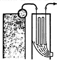
One adaptation of the separately fired superheater is the twin furnace. It consists of two furnaces in one unit. Superheater tubes are placed in one furnace and the steam from both pass through it.
