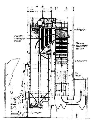
Here steam generation is largely by radiant energy transfer—there are no boiler convection sections.
