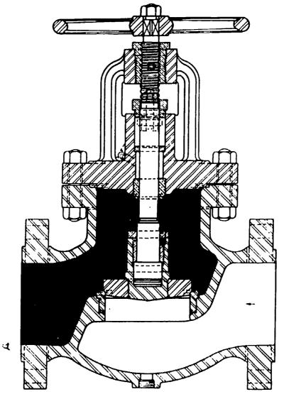
Globe Type Outside-Screw-and-Yoke Stop Valve (Schutte and Koesting Co.)
