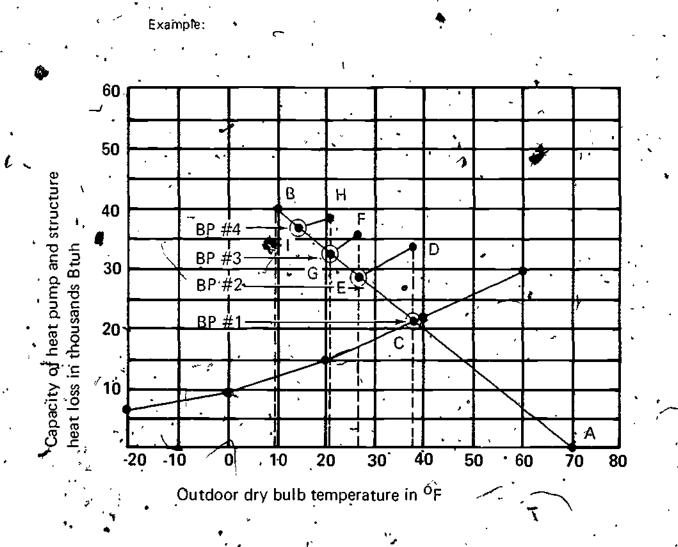
Procedure for sizing a heat pump on the cooling load
