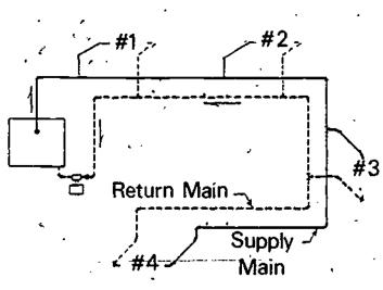
Two Pipe Direct Return Forced Hot Water Heating System
