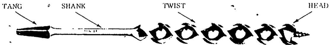
Fig. E-29. Parts of an auger bit
