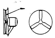
Figure 8. Propeller fan.
