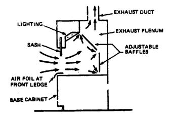
Figure 4. Standard laboratory fume hood.
