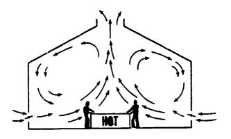
cause of its lower density (weight), and if openings are provided in the roof, the hot air passes out into the atmosphere. As the rising air leaves, fresh air flows into the building through openings near ground level to replace the discharged air. This flow is illustrated in Figure 1. The amount of air that is dis-
