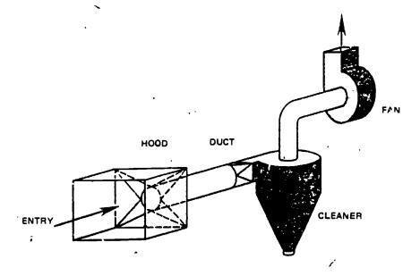
Figure 2. Elements of a local exhaust system.
