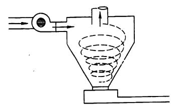
Figure 11. Cyclone collector.
