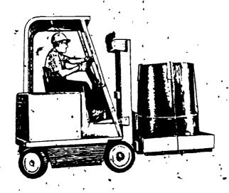
Figure 8. Industrial truck with platform.
