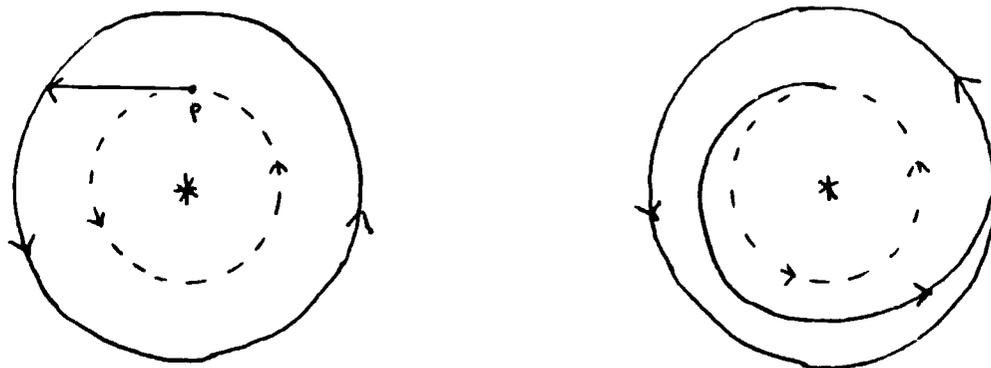
Neither of these situations allows the ship to return to  $p$ , as it must, since undeflected orbits always close. (The orbit is undeflected after the thrust.) By the way, the new orbit must go outside the old one for any number of reasons. You can say "more energy" or simply note that with an increased velocity gravity does not have enough time to change the velocity as much as before; the orbit at that point must bend less away from a straight line.
