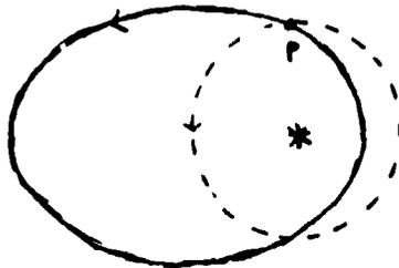
since, in this orbit, the new velocity at the point of thrust obviously points slightly away from the earth (it must in order to cross the old orbit).
