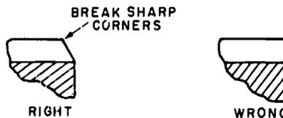
The ends of the coating must be finished off so that there is no load on any edge of the sprayed coating when the part is put back in service.
