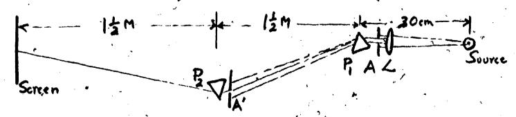
With the layout approximately as shown, the length of the spectrum at the second aperture, 'A' will be about 6 cm. and width about 2 cm. (Aperture A about 6 mm. less). A' should be an adjustable slit, with
