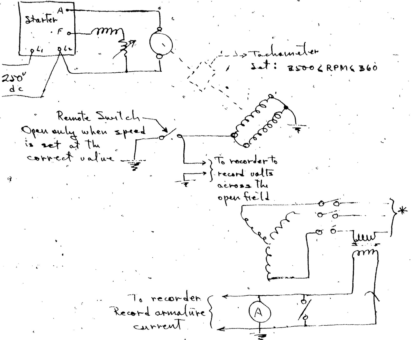
Lab Connection for Determining  $X_g$  by the "Slip Test"
