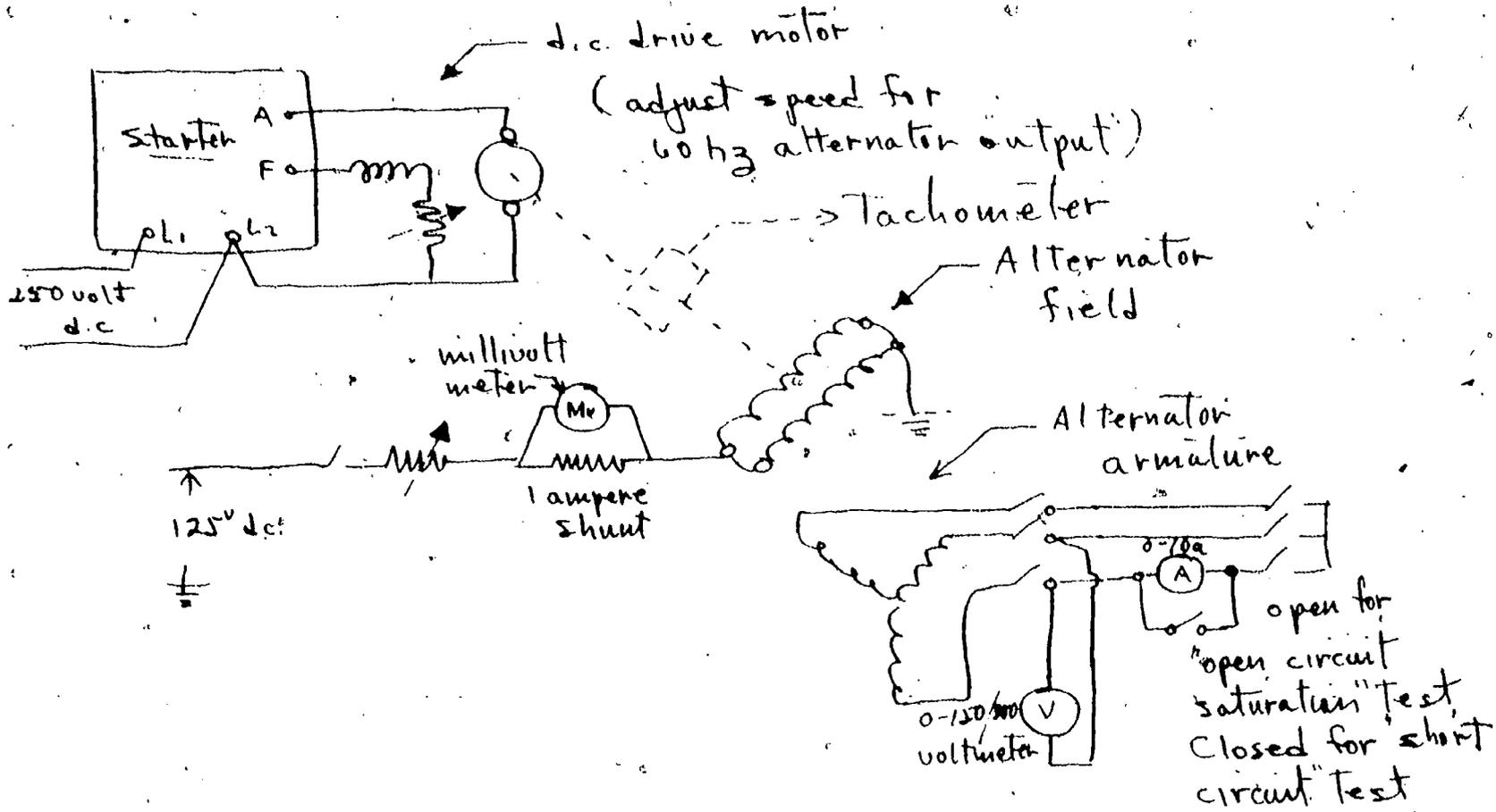
Note - reduce field current of the alternator to its minimum value, and short around the ammeter before short circuiting the alternator
