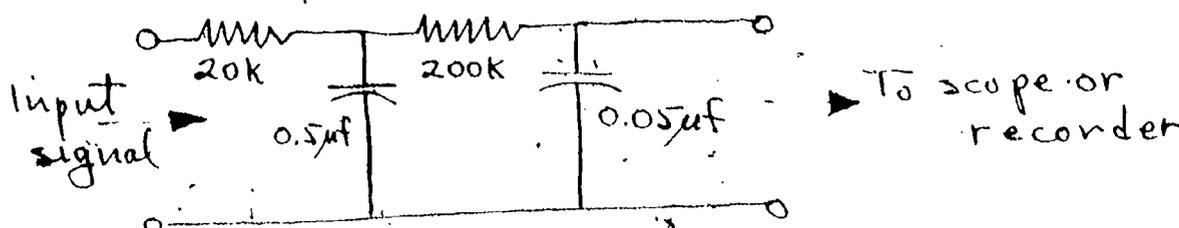
NOTE: If a voltmeter read-out is used, the input impedance must be greater than 20K ohms per volt. Appropriate ranges are 0-1.5/0-5 volt d.c. The black terminal may be connected to the lab ground to reduce pick-up.
