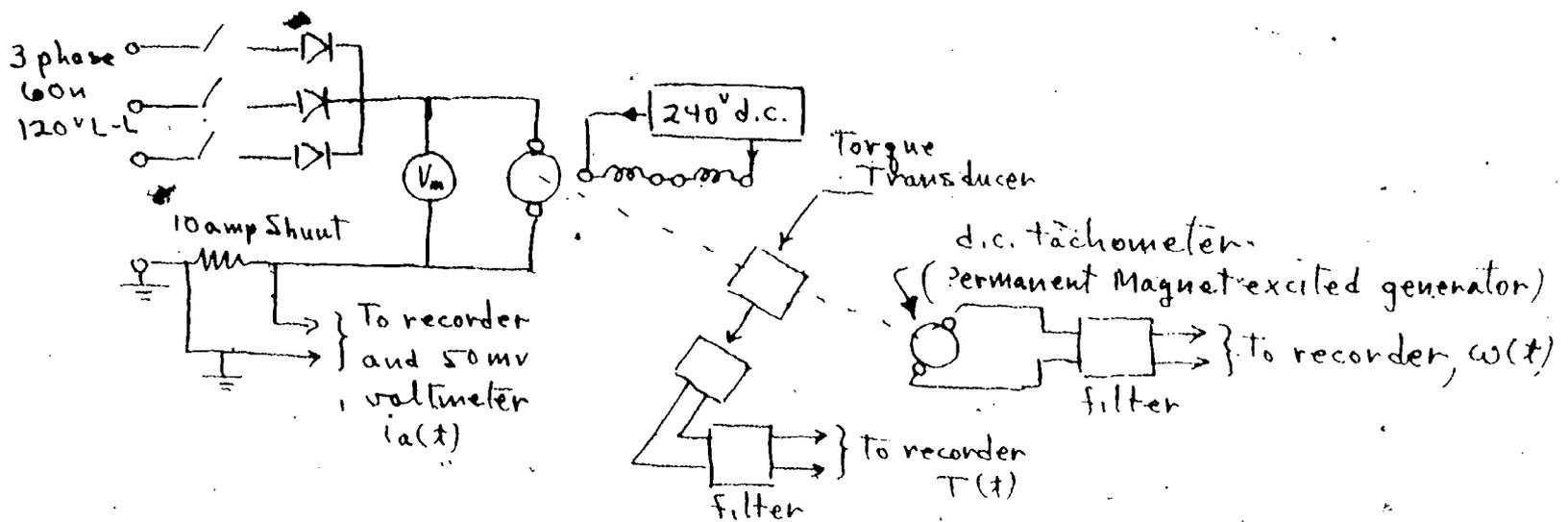
At  $t=0$ , with all resistance removed from the field of the motor, close the rectifier supply switch and record  $\omega(t)$ ,  $i_a(t)$ ,  $T(t)$ , and  $V_{d.c.}$ . Plot both the experimental and theoretical results on the same sheet; account for discrepancies.
