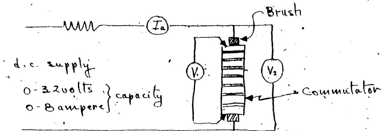
$V_1$  - measures voltage drop across armature copper
