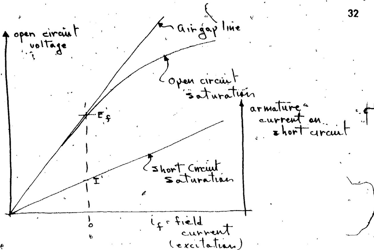
The short circuit saturation curve is obtained by driving the machine being tested at rated speed with the armature short circuited and recording armature and field current for field current values over the range from zero to 125-150% of rated value. Note that readings are taken for short circuit currents in the steady state, i.e., after any transients associated with the change in  $i_f$  have decayed out.
