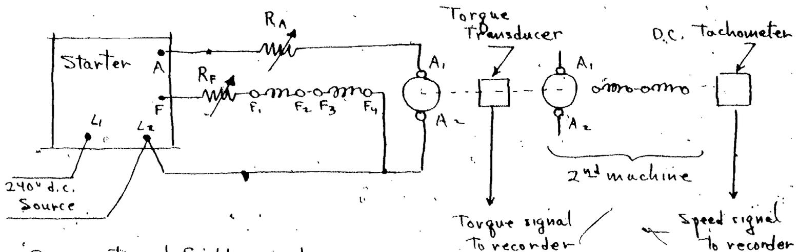
$R_F$  - external field resistor
