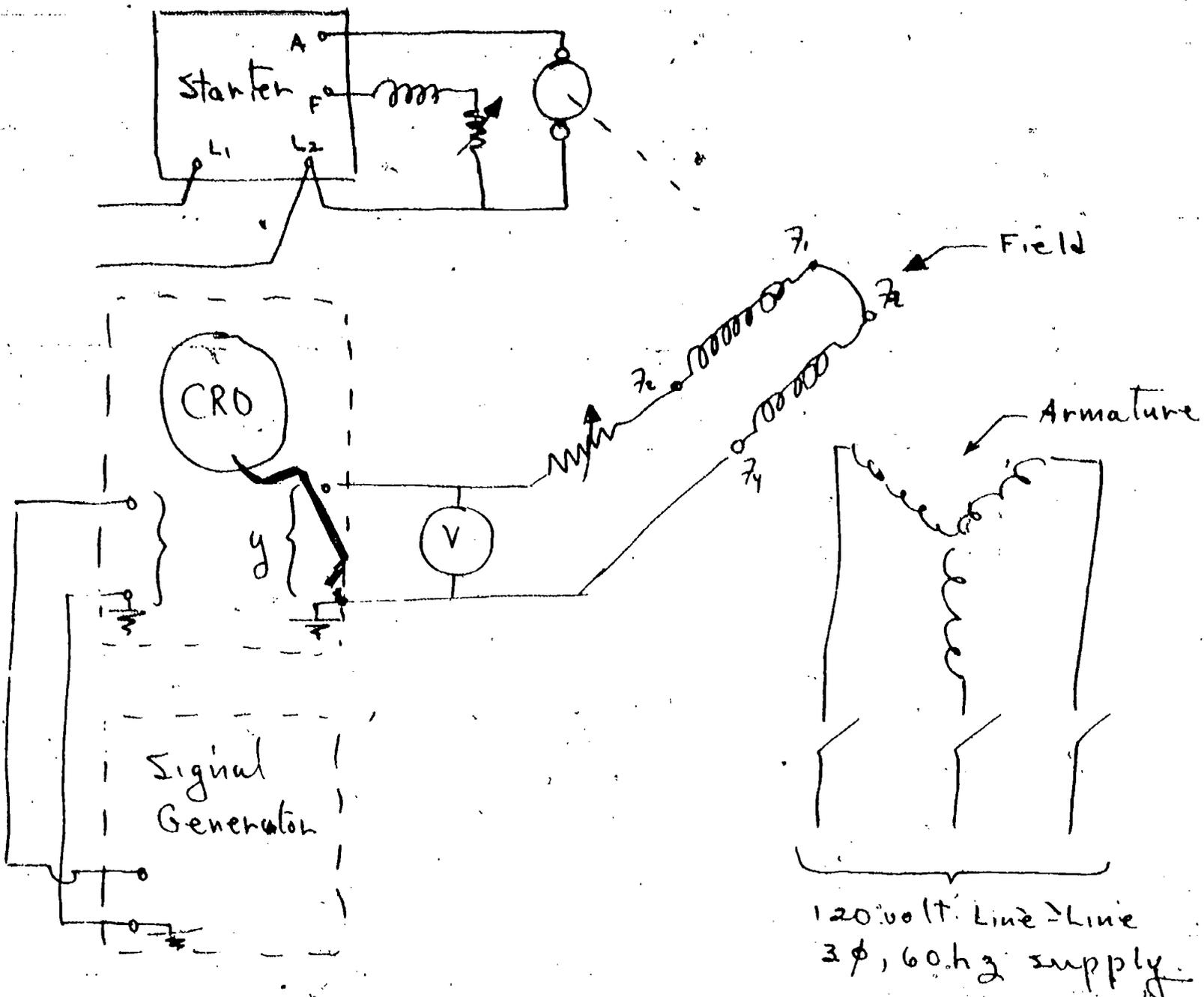
Lab Connections for Frequency Changer Operation
