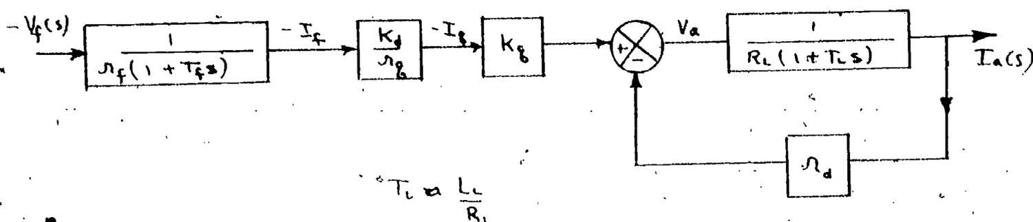
The transfer function for the Amplidyne is, from the block diagram:
