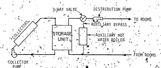
Figure 8-4. Liquid System for Solar Space Heating with Auxiliary Boiler
