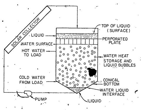
Figure 22-4. Direct Contact Liquid-Liquid Heat Exchanger
