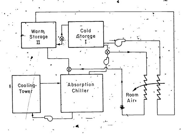
Figure 10-3. Alternative Cooling Subsystem with Two Cooling Coils
