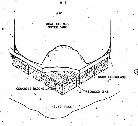
Figure 6-2. Bottom Insulation and Support Scheme for Water Storage Tanks
