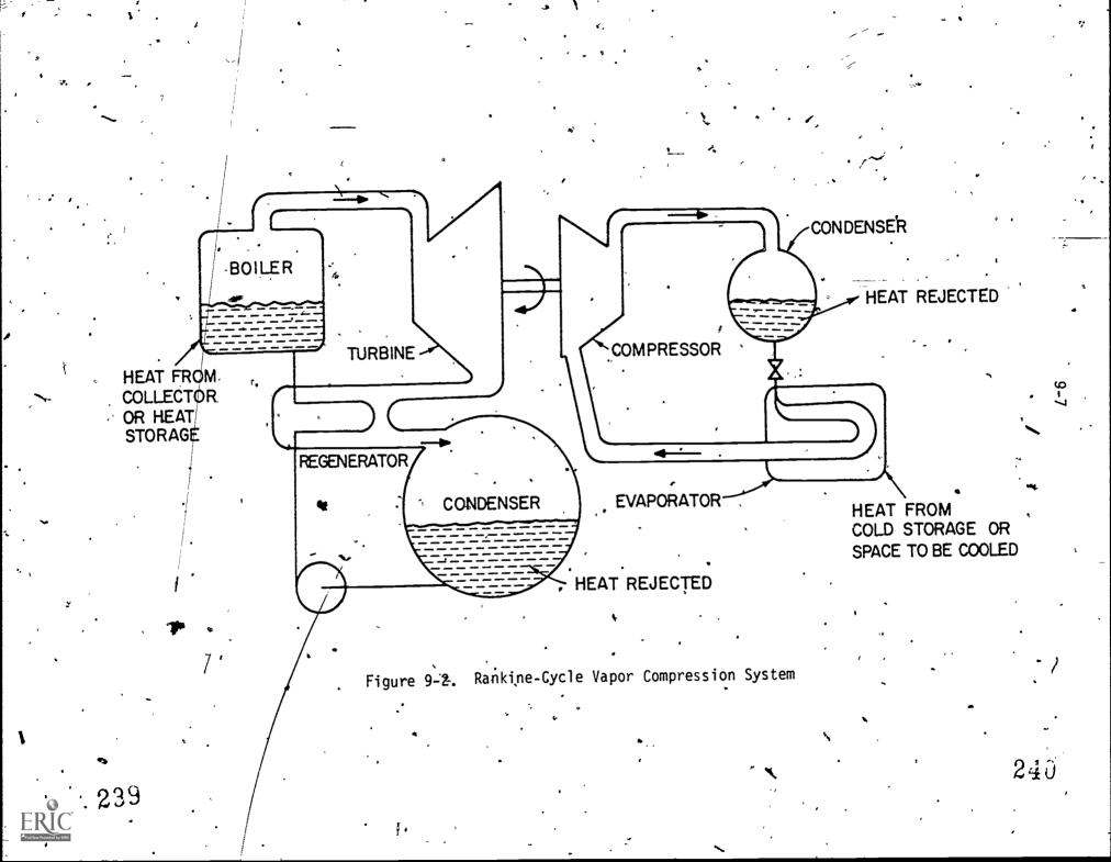
liquid in the condenser and is pumped back to the boiler. The regenerator is a heat exchanger to recover some of the heat from the vapor ejected from the turbine. This machine is still in the experimental and developmental stages and is not yet available as an operational unit.
