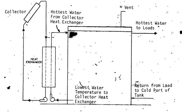
Figure 6-1. Operation of a Water Heat Storage Tank
