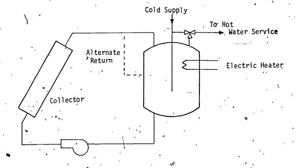
Figure 7-2. Direct Heating, Pump Circulation Type of Solar Water Reater
