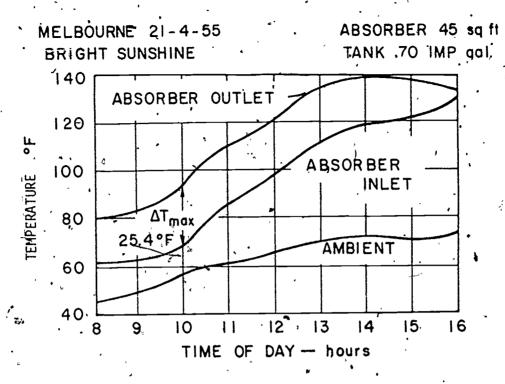
Figure 7-8. Absorber and Tank Temperatures for Thermosiphon Flow During a Typical Day
