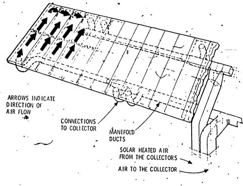
gure 5-8. Typical Arrangement of Internally Manifolded Collector Modules in an Array factor in any scheme is to be sure that joints in the duct system do not leak.
