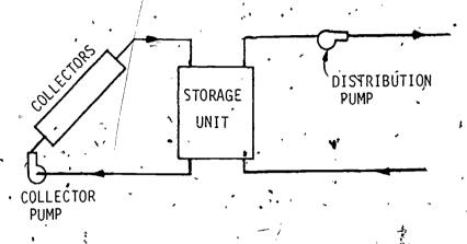
Figure 8-2. Water System Arrangement for Solar Space Heating
