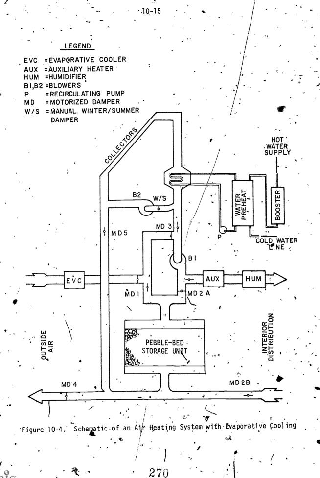
delivered to the top of the gravel bed, and discharged at the bottom. In a distance of two to three feet in the direction of air travel, all of the heat in the air is transferred to the rocks. To provide for adequate heat storage during the day, the depth of the rock bed should be about five to six feet.
