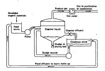
Figure 19 Concept of a unit for continuous conversion of organic material to methane by anaerobic fermentation (without oxygen).
