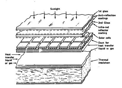
Figure 15 Co.nbination collector arrangement to extract both electrical and heat energy from sunlight.
