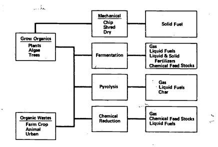
Figure 18 Various methods of producing different kinds of fuels from solar energy.
