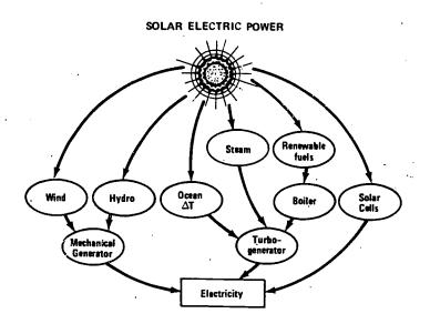
Figure 10 This diagram shows the various routes by which solar energy can be converted to electricity.
