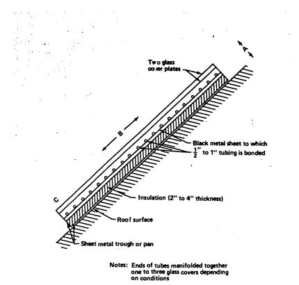
Dimensions: Thickness (A direction). 3 inches to 6 inches Length (B direction) 4 feet to 20 feet Width (C direction) 10 feet to 50 feet Slope dependent on location and on wintersummer load comparison
