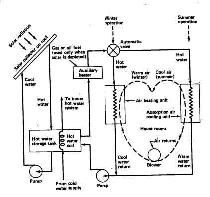
Figure 8 This diagram shows a system that combines residential heating and cooling with solar energy.
