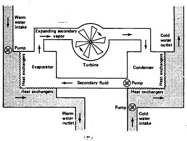
Figure 17 Diagram of a closed cycle ocean thermal power plant.
